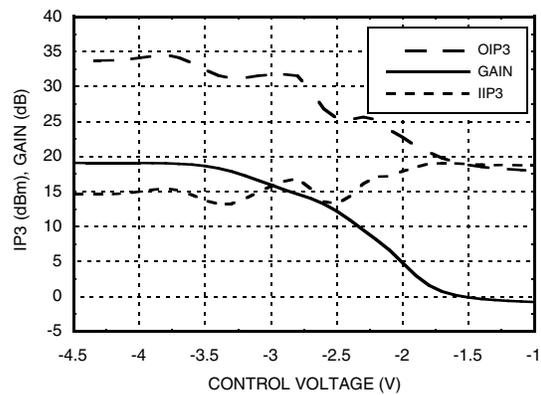
**IP3 and Gain @ 10 GHz, Pin = -10 dBm**
