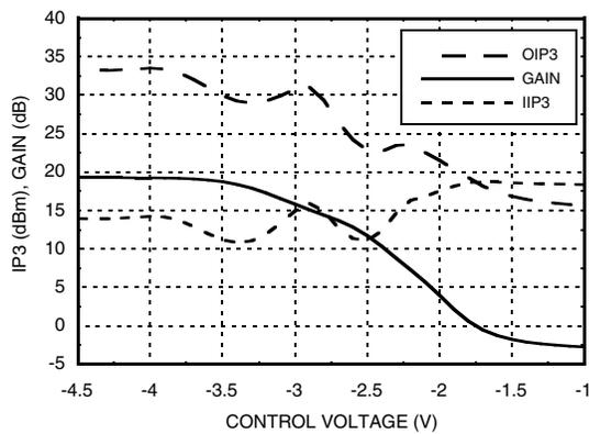
**IP3 and Gain @ 8 GHz, Pin = -10 dBm**
