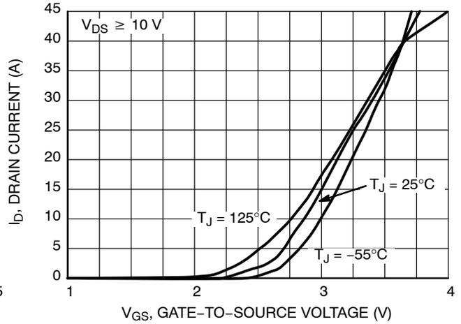
Figure 2. Transfer Characteristics
