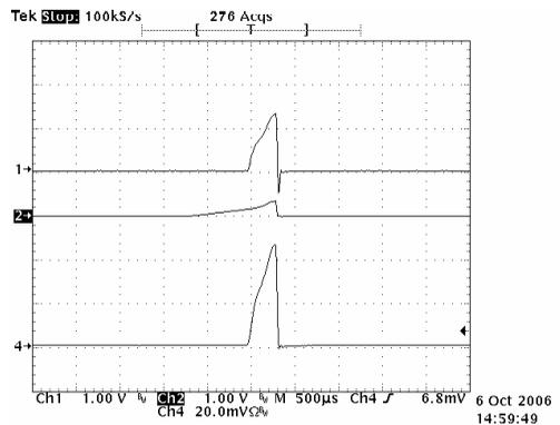
Short Circuit Protection: CH1:  $V_{OUT}$ .
