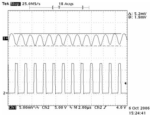
12Vin Output Ripple: CH1: V<sub>OUT</sub>.
