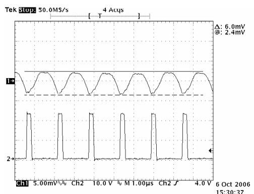
22Vin Output Ripple: CH1: V<sub>OUT</sub>.
