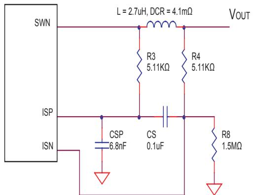
**Over-current detection circuit for  $I_{MAX} < \{60\text{mV} / \text{DCR}\}$**
