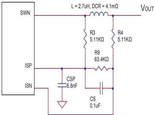
**Over-current detection circuit for  $I_{max} > 60\text{mV} / \text{DCR}$**
