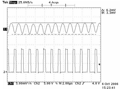
12Vin Output Ripple: CH1:V<sub>OUT</sub>. CH2:
