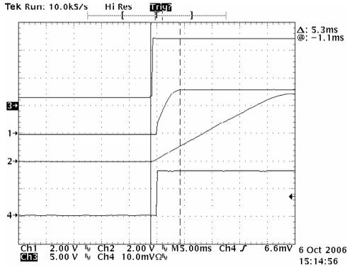
Start-up in to 3A Load: CH1:V<sub>OUT</sub>.
