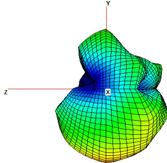
**FIGURE 4.6.7 3D RADIATION PATTERN OF ANTENNA AT 6000MHZ BAND OF PORT 2 IN FREE SPACE**
