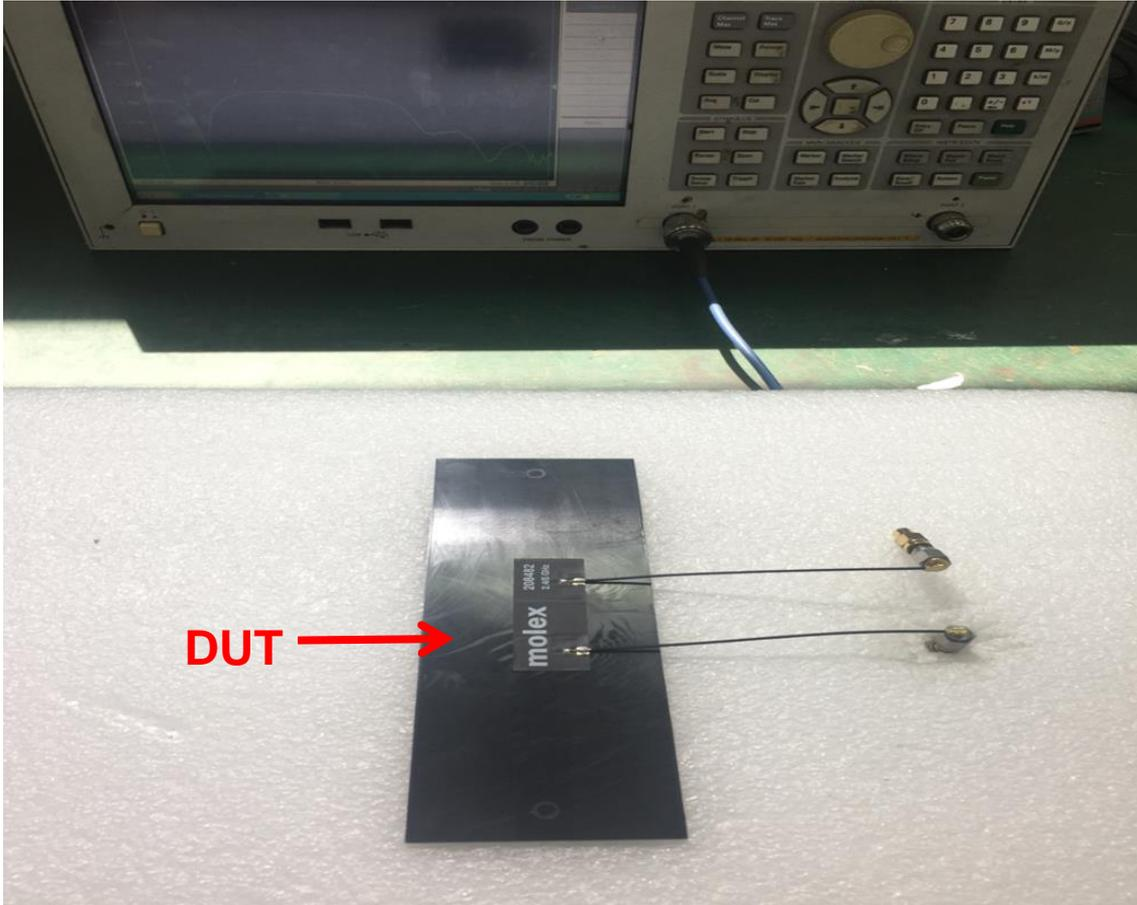
**FIGURE4.1.2 ANTENNA LOADED WITH PC/ABS BLOCK OF 1.5MM THICKNESS TESTED WITH VNA E5071C**
