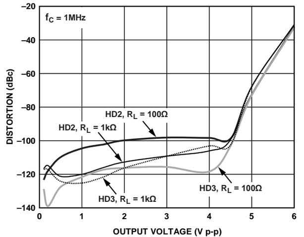
Figure 19. Distortion vs. Output Voltage for Various Loads
