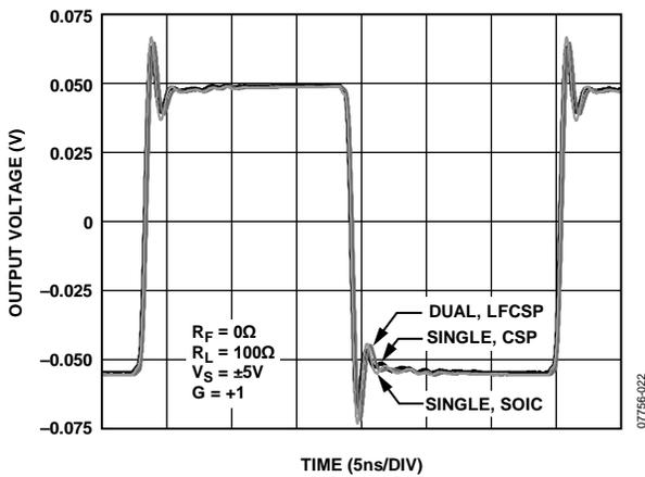
Figure 20. Small Signal Transient Response vs. Package
