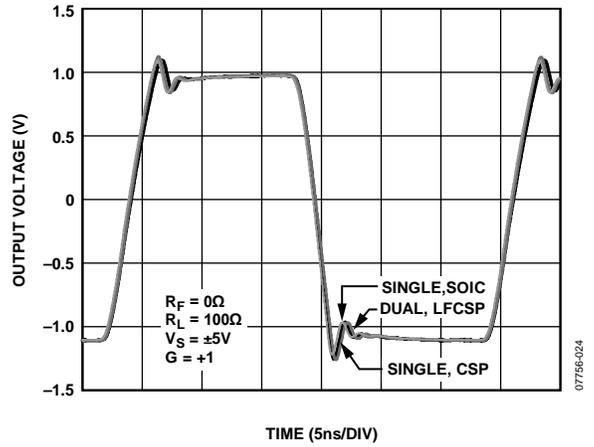
Figure 23. Large Signal Transient Response vs. Package
