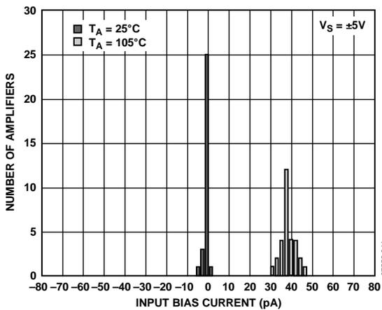
Figure 40. Input Bias Current Histogram over Temperature
