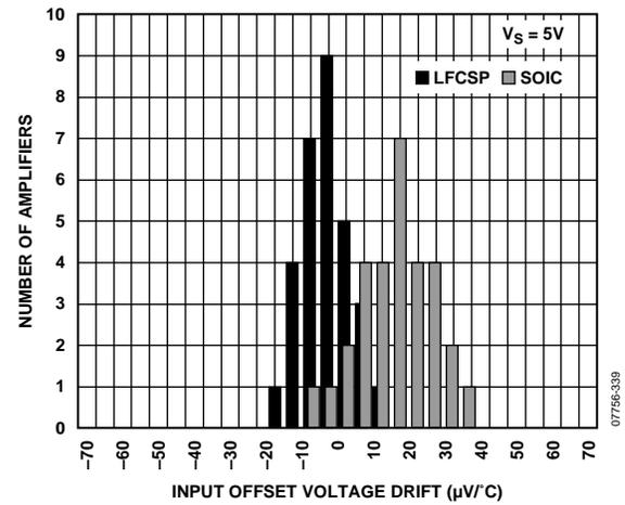
Figure 42. Input Offset Voltage Drift Histogram
