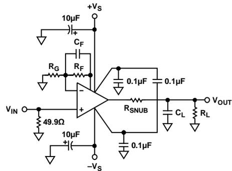
Figure 56.  $R_{SNUB}$  or  $C_F$  Used to Reduce Peaking
