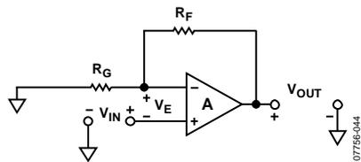
Figure 52. Noninverting Configuration
