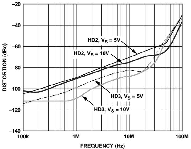
Figure 16. Distortion vs. Frequency for Various Supplies, G = 2, V<sub>OUT</sub> = 2 V p-p
