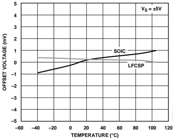
Figure 38. Offset Voltage vs. Temperature
