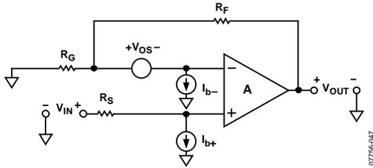
Figure 55. DC Errors of the Voltage Feedback Amplifier
