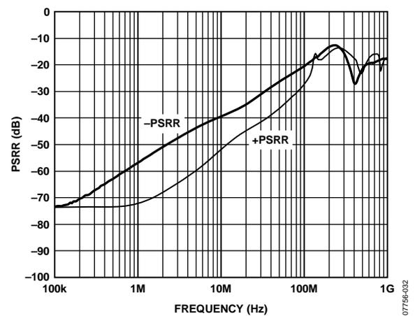
Figure 25. Power Supply Rejection Ratio (PSRR) vs. Frequency
