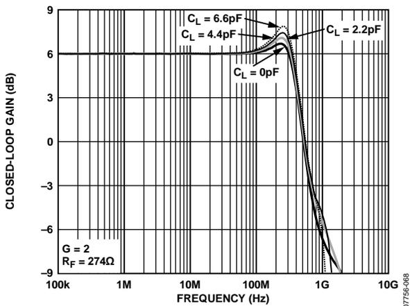
Figure 10. Small Signal Frequency Response for Various  $C_L$
