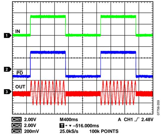
Figure 58. Power-Down Operation
