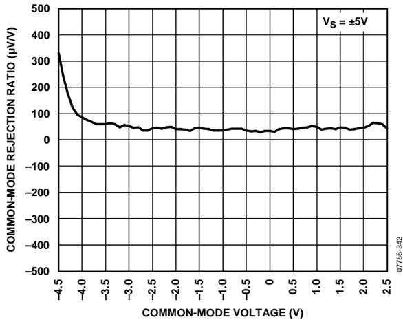
Figure 44. Common-Mode Rejection vs. Common-Mode Voltage,  $V_S = \pm 5V$
