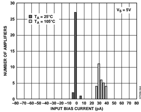
Figure 43. Input Bias Current Histogram over Temperature
