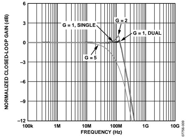
Figure 11. Large Signal Frequency Response for Various Gains
