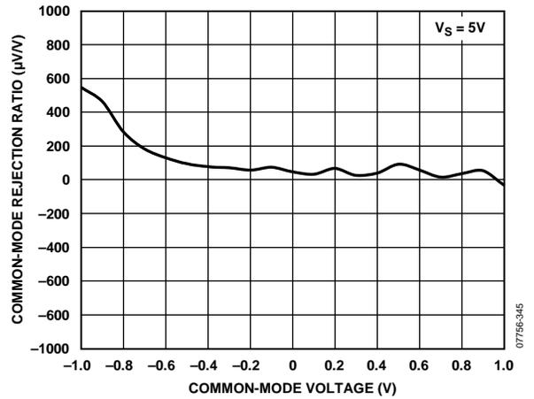
Figure 45. Common-Mode Rejection vs. Common-Mode Voltage,  $V_S = 5V$
