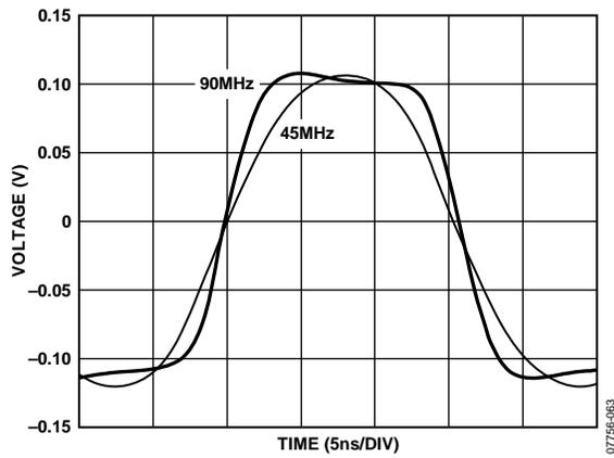
Figure 69. Small Signal Transient Response (Low-Pass Filter)
