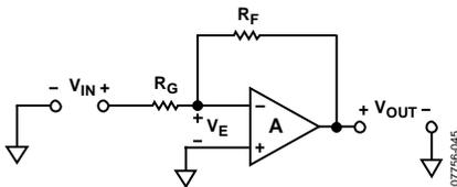
Figure 53. Inverting Configuration
