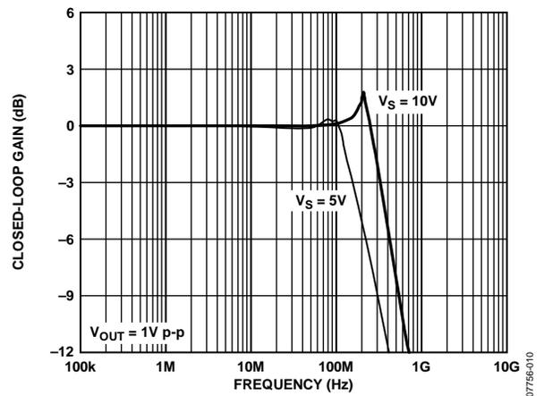
Figure 12. Large Signal Frequency Response for Various Supplies
