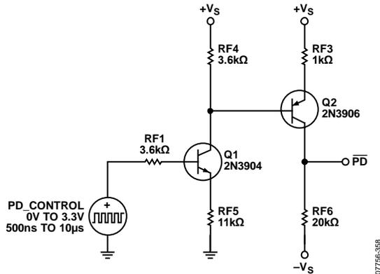
Figure 57. Power-Down Circuit
