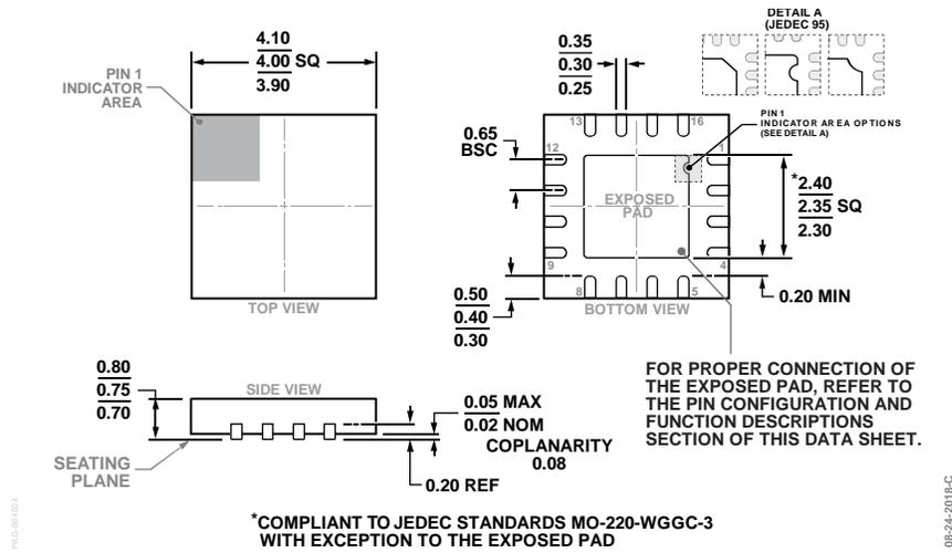
Figure 73.16–Lead Lead Frame Chip Scale Package [LFCSP]
