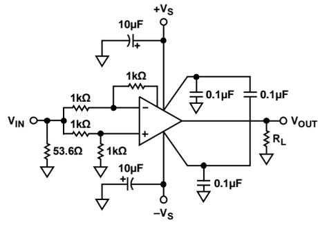
Figure 51. Common-Mode Rejection
