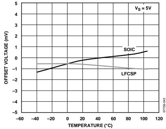
Figure 41. Offset Voltage vs. Temperature
