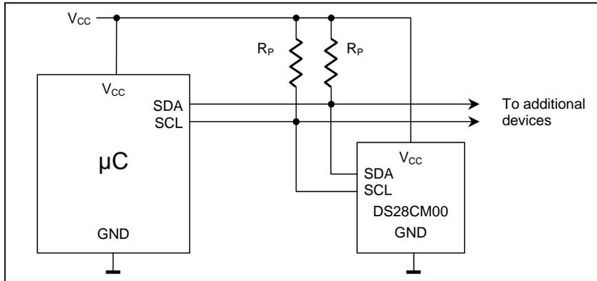
For I<sup>2</sup>C systems, the rise time and fall time are measured from 30% to 70% of the pullup voltage. The maximum bus capacitance  $C_B$  is 400pF. The maximum rise time must not exceed 300ns. Assuming maximum rise time, the maximum resistor value at any given capacitance  $C_B$  is calculated as:  $R_{P_{MAX}} = 300ns / (C_B * \ln(7/3))$ . For a bus capacitance of 400pF the maximum pullup resistor would be 885Ω.
