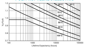
Vw = Working DC Voltage • Vn = Rated DC Voltage
