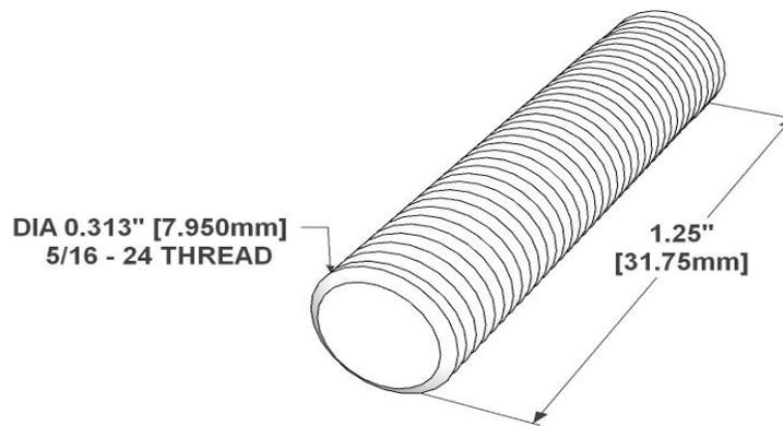
All measurements are in inches [millimeters]
