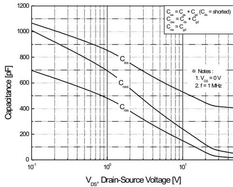
Figure 5. Capacitance Characteristics
