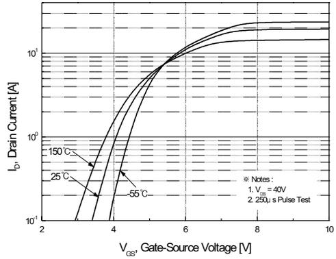
Figure 2. Transfer Characteristics
