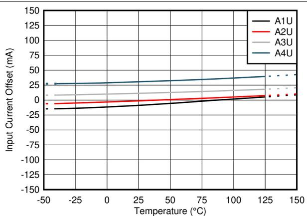
**Figure 7-4. TMCS1101AxU Input Offset Current vs Temperature**
