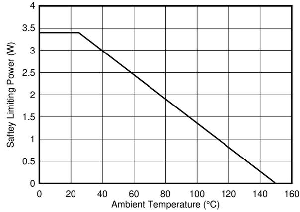
**Figure 7-30. Thermal Derating Curve for Safety-Limiting Power**
