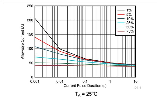
**Figure 8-6. Maximum Repetitive Pulsed Current vs. Pulse Duration**
