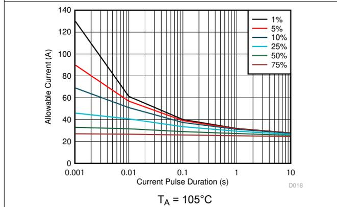
**Figure 8-8. Maximum Repetitive Pulsed Current vs. Pulse Duration**
