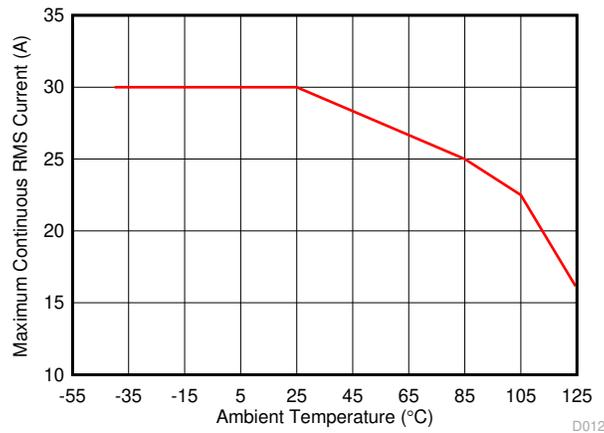
**Figure 8-5. Maximum Continuous RMS Current vs. Ambient Temperature**
