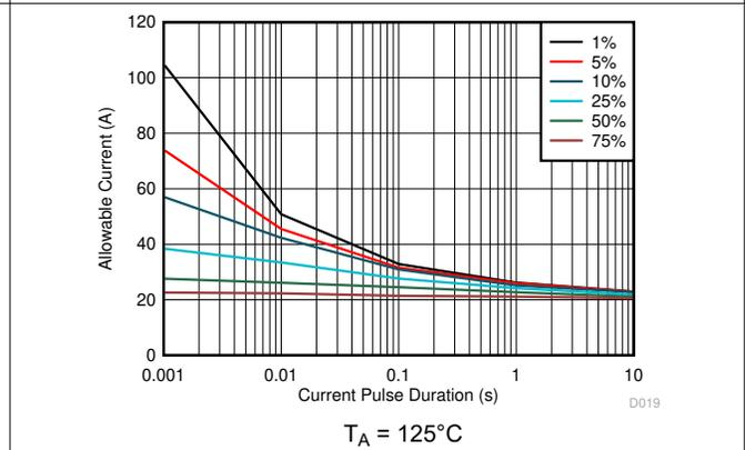
**Figure 8-9. Maximum Repetitive Pulsed Current vs. Pulse Duration**
