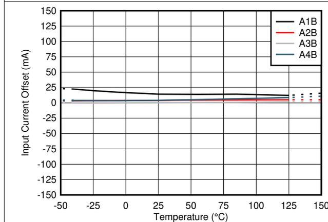
**Figure 7-3. TMCS1101AxB Input Offset Current vs Temperature**
