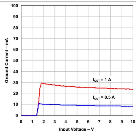
Figure 6. Ground Current vs Input Voltage
