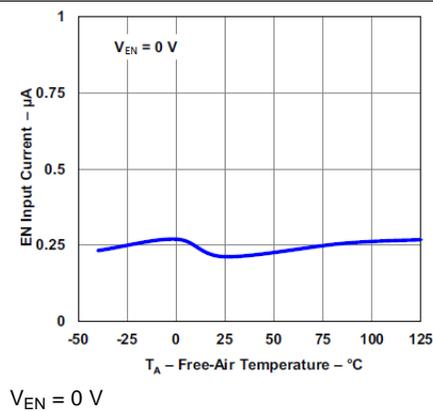
Figure 9. EN Input Current vs Temperature
