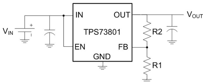
Figure 24. Adjustable Operation
