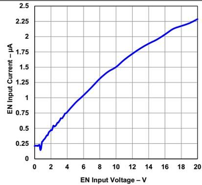
Figure 10. EN Input Current vs EN Input Voltage
