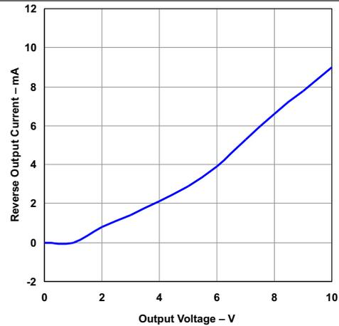
$T_J = 25 \text{ }^\circ\text{C}$        $V_{IN} = 0 \text{ V}$
