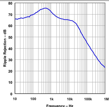
$V_{IN} = 2.7 \text{ V}$        $V_{RIPPLE} = 0.05 \text{ V}_{PP}$        $I_{OUT} = 750 \text{ mA}$
