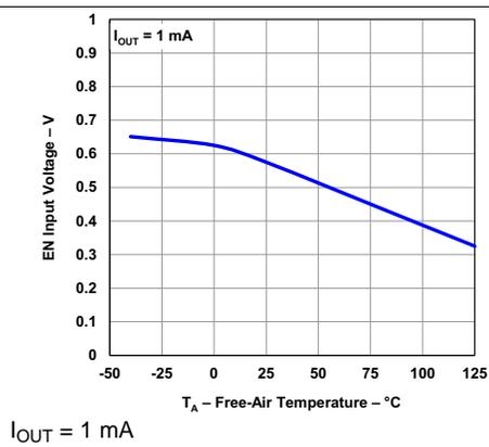
Figure 12. EN Threshold (On to Off) vs Temperature
