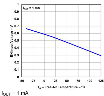
Figure 11. EN Threshold (Off to On) vs Temperature
