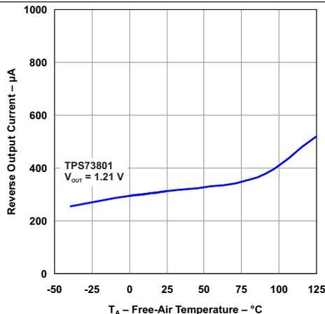
$V_{IN} = 0 \text{ V}$
