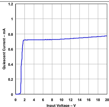
Figure 5. Quiescent Current vs Input Voltage
