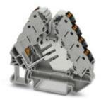
Potential distributors, Nom. voltage: 250 V, Nominal current: 17.5 A, Cross section: 0.14 mm² - 2.5 mm², AWG: 12 - 26, Connection type: Push-in connection, Width: 8.3 mm, Length: 64 mm, Color: gray, Assembly: NS 35/7,5, NS 35/15
