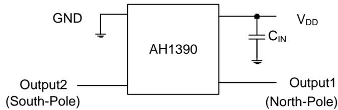
Note: 4.  $C_{IN}$  is for power stabilization and to strengthen the noise immunity, the recommended capacitance is 100nF typical and should be placed as close to the supply pin as possible.
