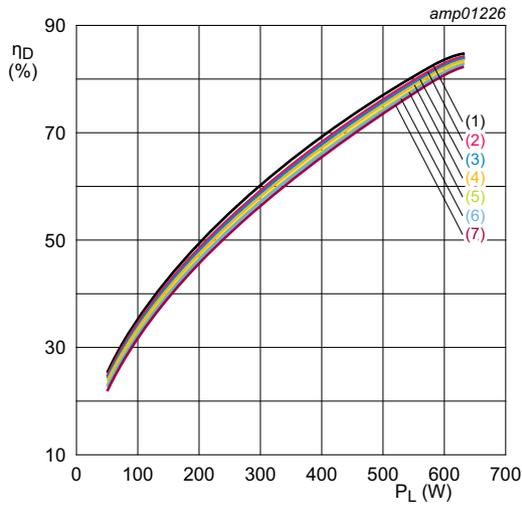
$V_{DS} = 50 \text{ V}; f = 225 \text{ MHz}.$
