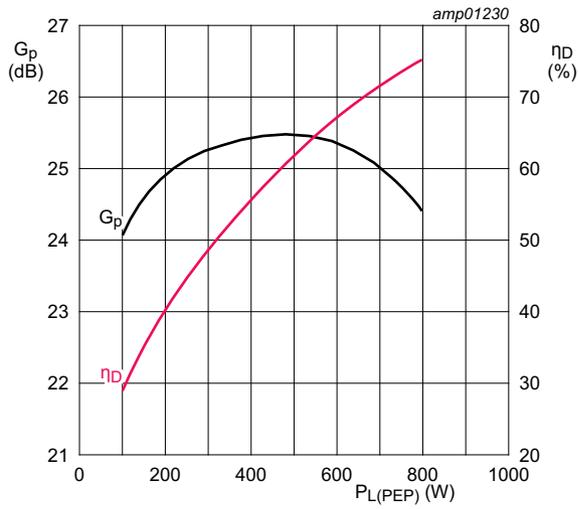
$V_{DS} = 50 \text{ V}; I_{Dq} = 2 \times 50 \text{ mA}; f_1 = 224.95 \text{ MHz}; f_2 = 225.05 \text{ MHz}.$
