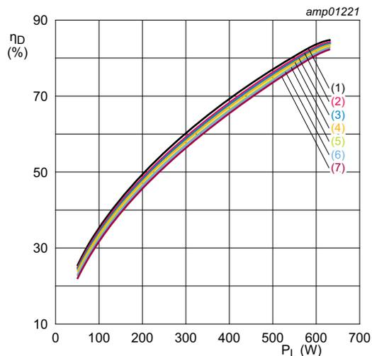
$V_{DS} = 50 \text{ V}; f = 225 \text{ MHz}; t_p = 100 \text{ }\mu\text{s}; \delta = 10 \text{ \%}$ .
