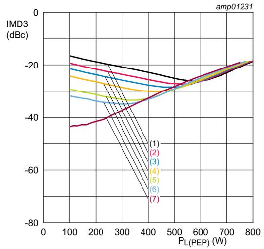
$V_{DS} = 50 \text{ V}; f_1 = 224.95 \text{ MHz}; f_2 = 225.05 \text{ MHz}.$
