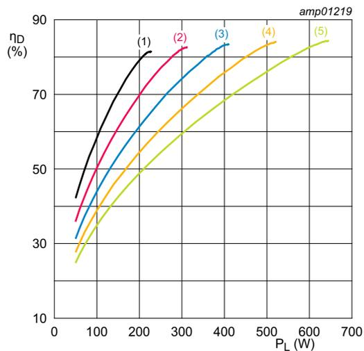
$I_{Dq} = 2 \times 50 \text{ mA}$ ;  $f = 225 \text{ MHz}$ ;  $t_p = 100 \text{ }\mu\text{s}$ ;  $\delta = 10 \text{ \%}$ .
