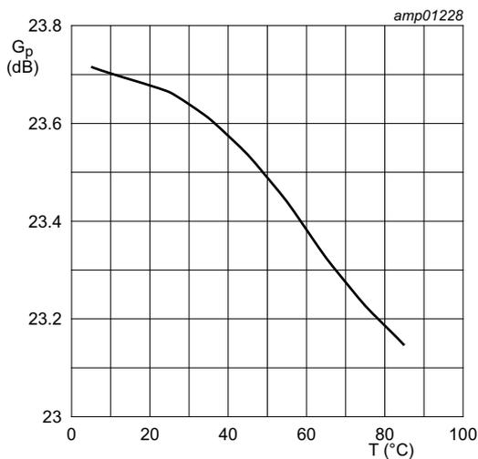
$V_{DS} = 50 \text{ V}; I_{Dq} = 2 \times 50 \text{ mA}; f = 225 \text{ MHz}; \text{ at } P_{L(2dB)}.$
