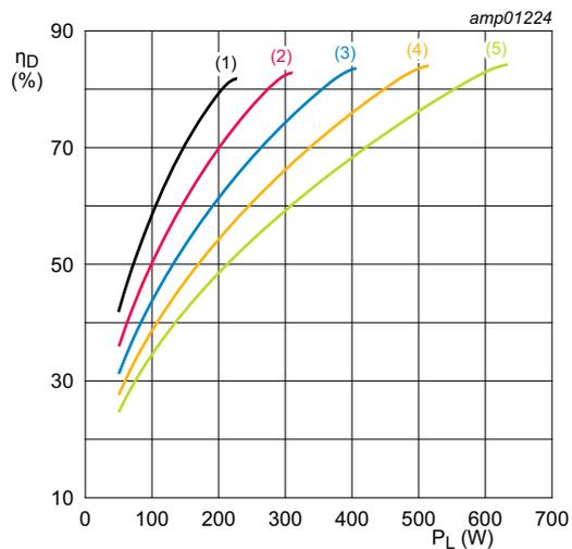
$I_{Dq} = 2 \times 50 \text{ mA}$ ;  $f = 225 \text{ MHz}$ .
