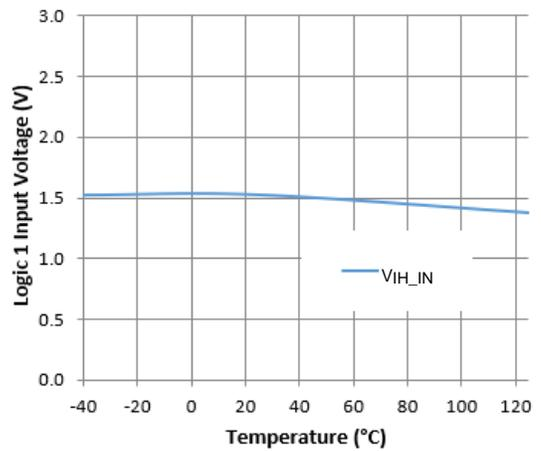
Figure 17. Logic 1 Input Voltage vs. Temperature
