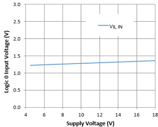
Figure 18. Logic 0 Input Voltage vs. Supply Voltage
