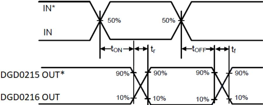
**Figure 1. Switching Time Waveform Definitions**
