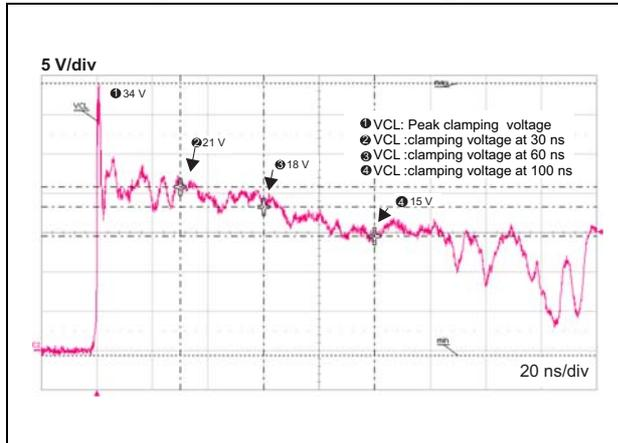
Figure 6. ESD response to IEC 61000-4-2 (-8 kV contact discharge)
