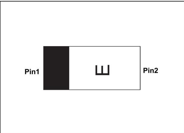
Note: The marking codes can be rotated by 90° or 180° to differentiate assembly location. In no case should this product marking be used to orient the component for its placement on a PCB. Only pin 1 mark is to be used for this purpose.
