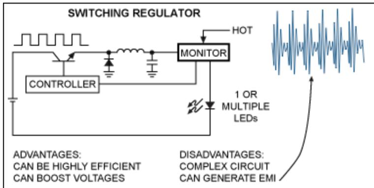
Figure 1b. In a basic switch-mode-regulation approach the main source of power loss comes from the energy dissipated by the current-sensing resistor. This design is highly efficient and can be reconfigured to boost voltages. It is, however, a more complex circuit and can generate EMI.
