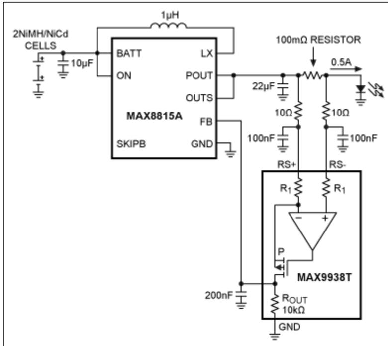
Figure 2. Working from Figure 1b, a current-sense amplifier such as the MAX9938T reduces the power losses in the current-sensing resistor to just a few tens of milliwatts vs. hundreds of milliwatts, or more, for the previous schemes in Figure 1.
