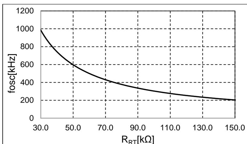
$$R_{RT} [\text{k}\Omega] = 34610 \times f_{osc} [\text{kHz}] ^{-1.023}$$
