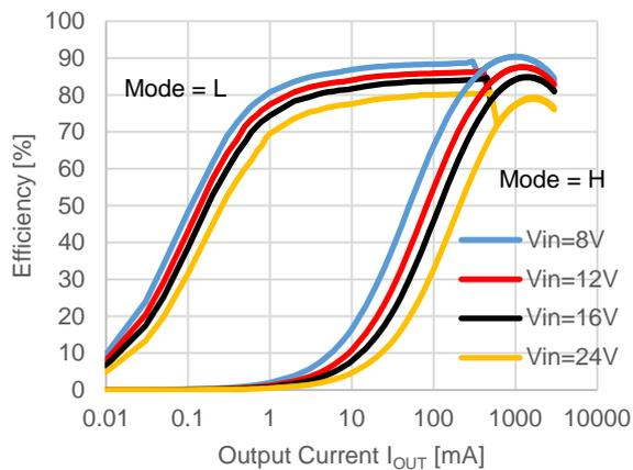
$V_{OUT} = 5.0\text{ V}$ ,  $f_{osc} = 250\text{ kHz}$
