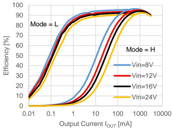
$V_{OUT} = 5.0\text{ V}$ ,  $f_{osc} = 500\text{ kHz}$
