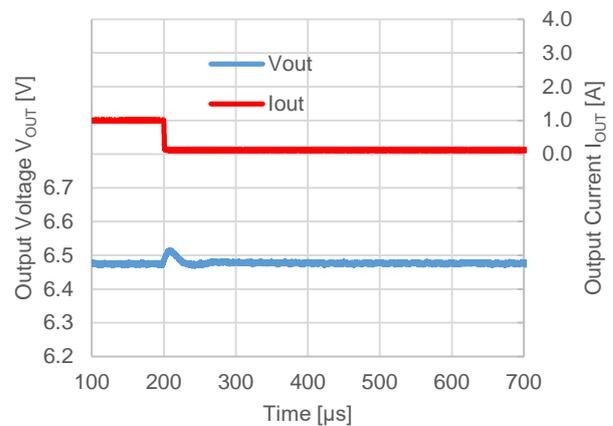
$V_{OUT} = 6.5\text{ V}$ ,  $V_{IN} = 12\text{ V}$ ,  $f_{OSC} = 500\text{ kHz}$
