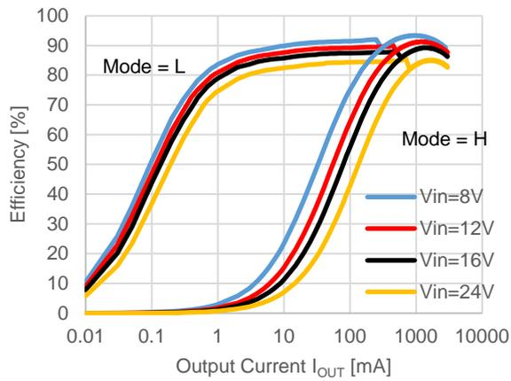
$V_{OUT} = 6.5\text{ V}$ ,  $f_{osc} = 250\text{ kHz}$
