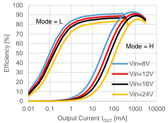
$V_{OUT} = 3.3$  V,  $f_{osc} = 1000$  kHz
