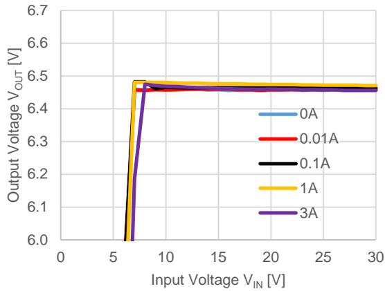
$V_{OUT} = 6.5\text{ V}$ ,  $f_{osc} = 500\text{ kHz}$ , Mode = H
