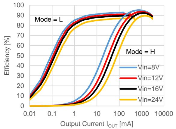
$V_{OUT} = 5.0\text{ V}$ ,  $f_{osc} = 1000\text{ kHz}$
