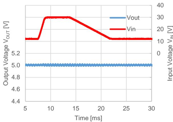
$f_{osc} = 250\text{ kHz}$ ,  $V_{IN} = 12\text{ V} \leftrightarrow 30\text{ V}$
