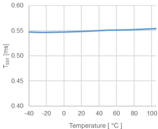
Externally Adjustable Soft-start Time (C<sub>SS</sub> = 4.7 nF)
