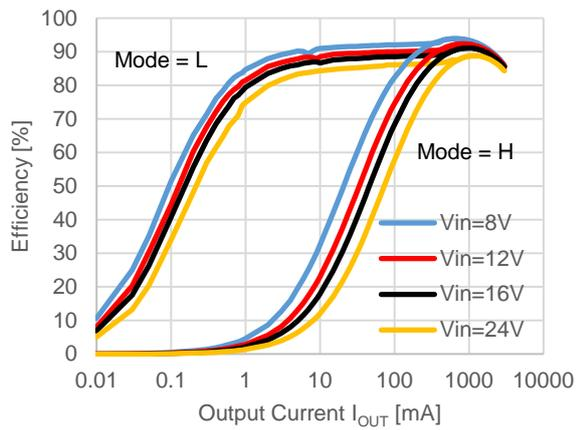
$V_{OUT} = 3.3$  V,  $f_{osc} = 500$  kHz
