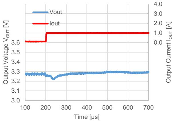
$V_{OUT} = 3.3\text{ V}$ ,  $V_{IN} = 12\text{ V}$ ,  $f_{OSC} = 500\text{ kHz}$
