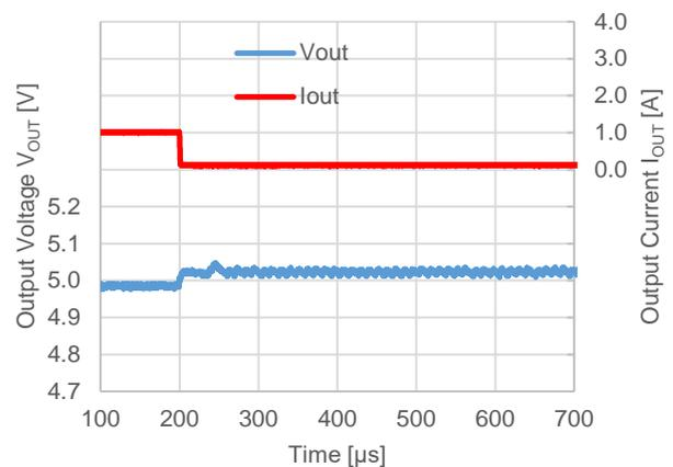
$V_{OUT} = 5.0\text{ V}$ ,  $V_{IN} = 12\text{ V}$ ,  $f_{OSC} = 500\text{ kHz}$
