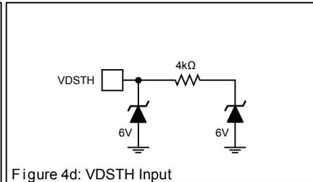
Figure 4d: VDSTH Input
