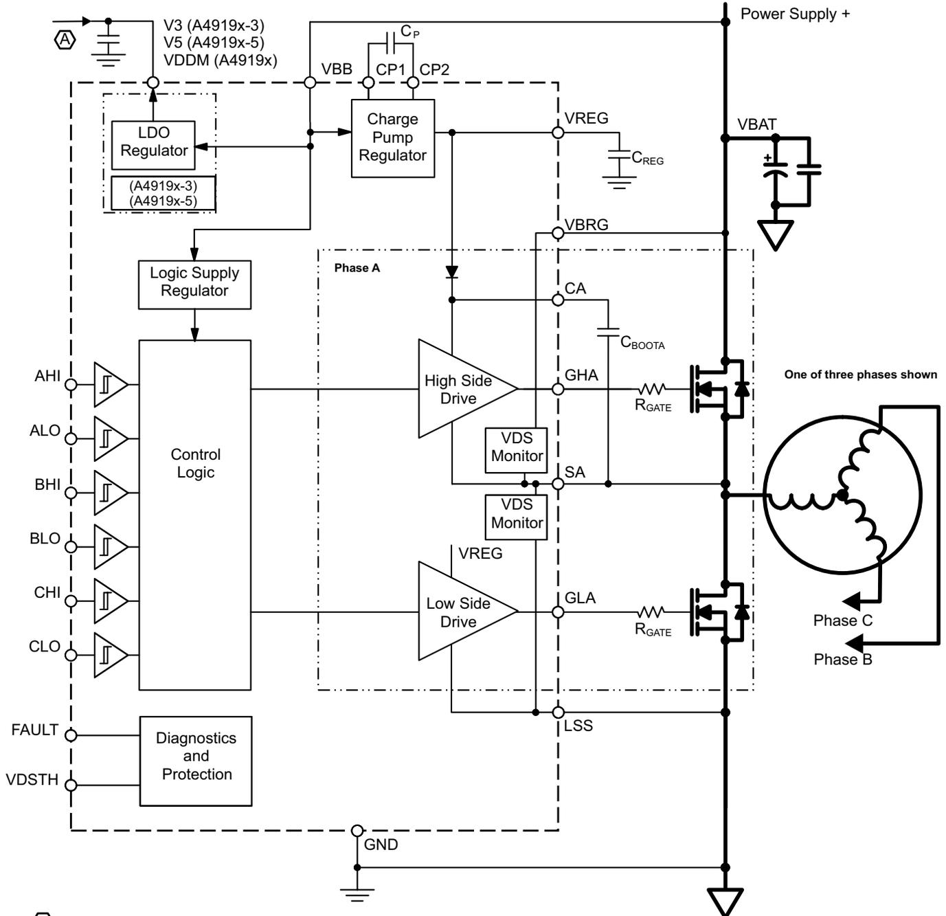
**(A)** External pin acts as a monitor input (VDDM) on variants without LDO regulator, and a supply voltage output on variants with LDO regulator (designated V3 or V5 for 3.3 V and 5.0 V variants respectively)
