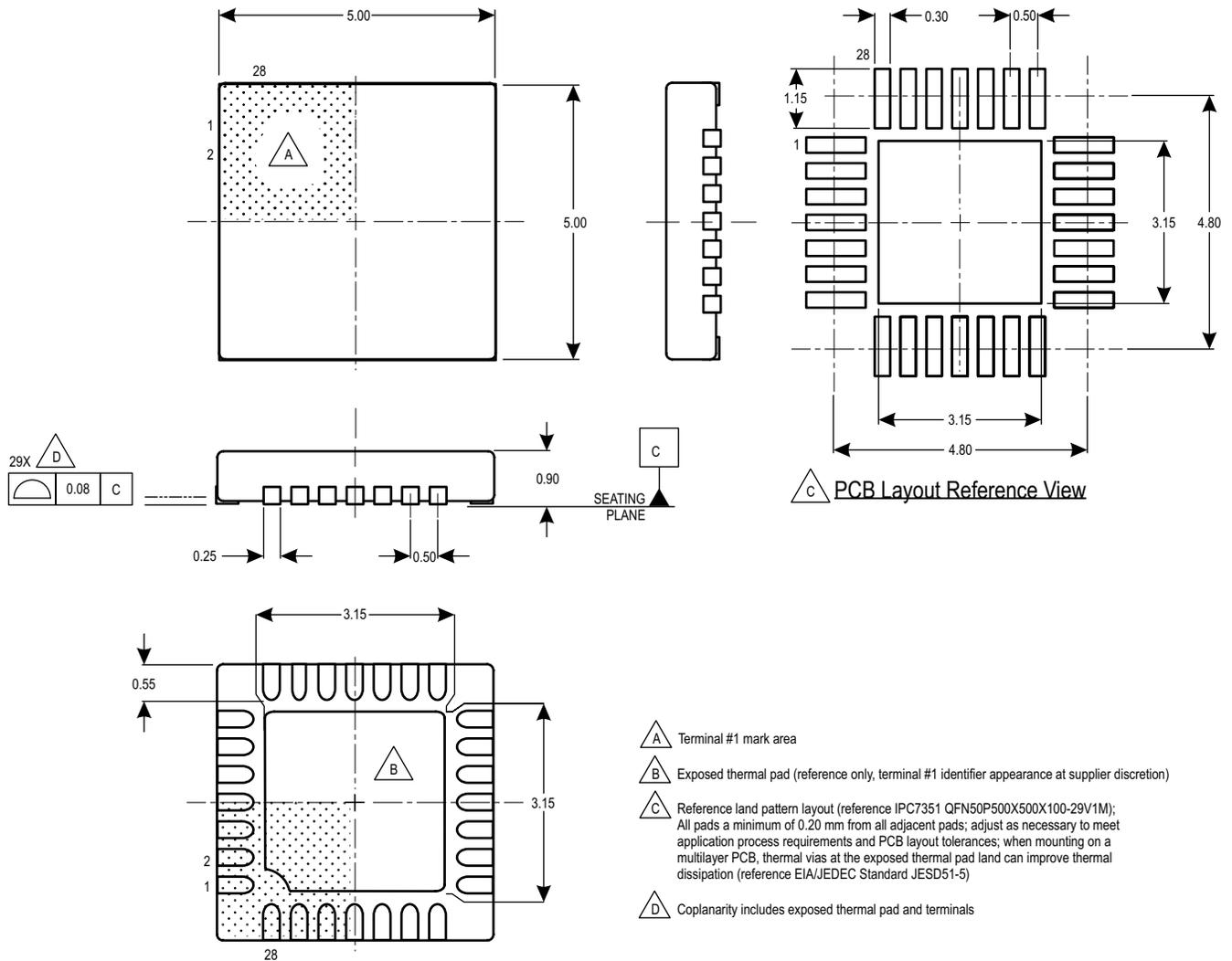
**Figure 7: Package ET, 28-Terminal QFN with Exposed Thermal Pad**
