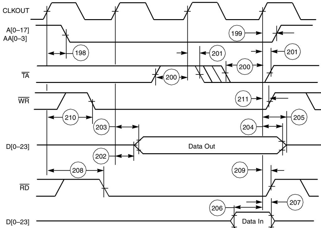
**Note:** Address lines A[0-17] hold their state after a read or write operation. AA[0-3] do not hold their state after a read or write operation.
