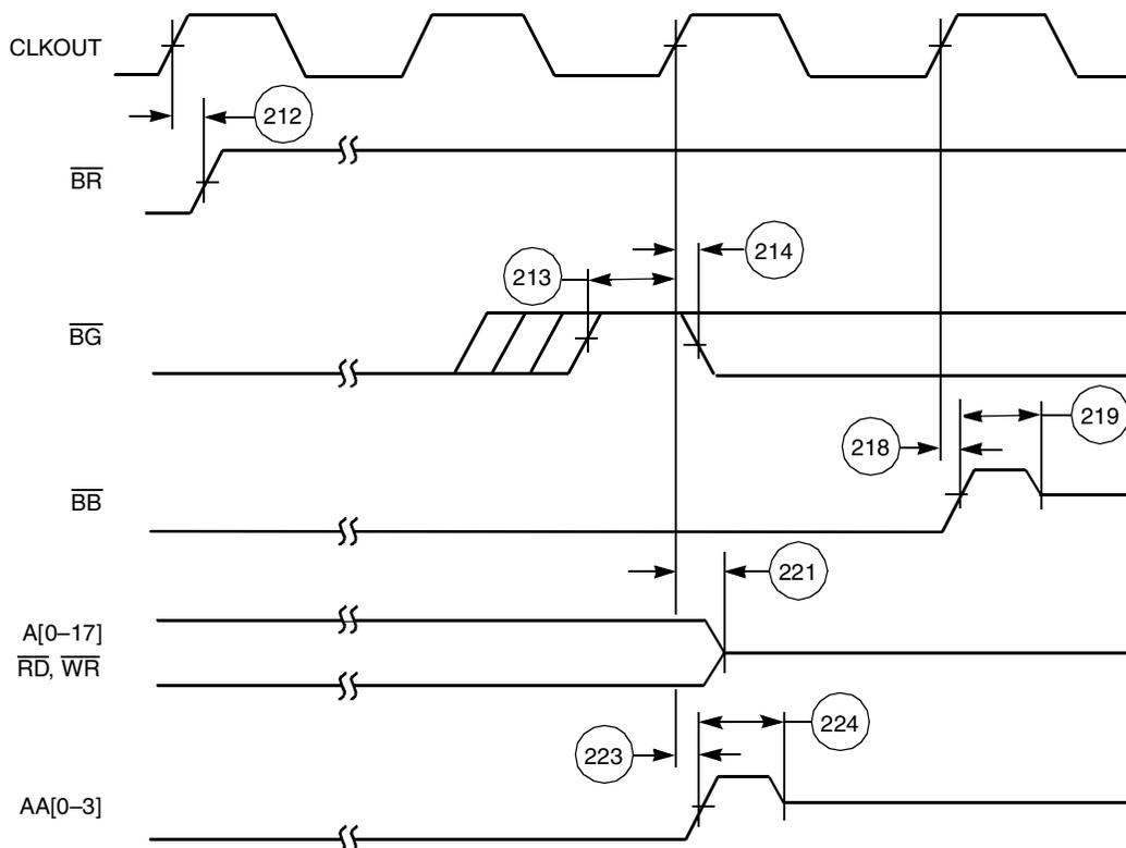
**Note:** Address lines A[0–17] hold their state after a read or write operation. AA[0–3] do not hold their state after a read or write operation.
