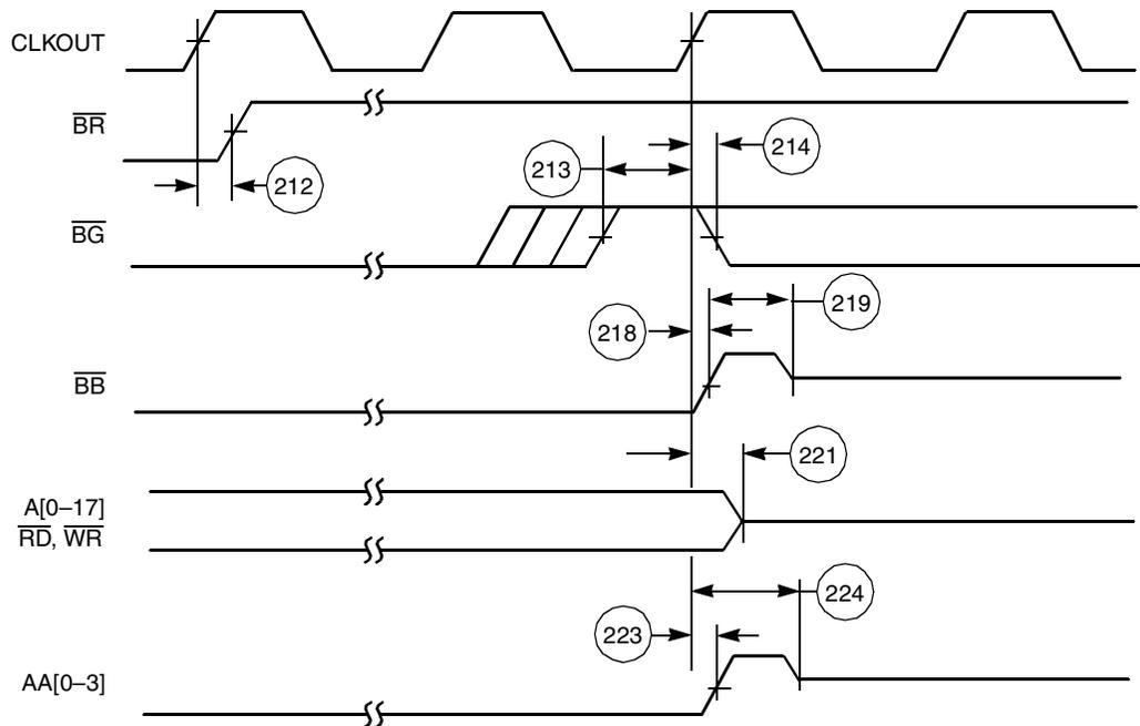
**Note:** Address lines  $A[0-17]$  hold their state after a read or write operation.  $AA[0-3]$  do not hold their state after a read or write operation.
