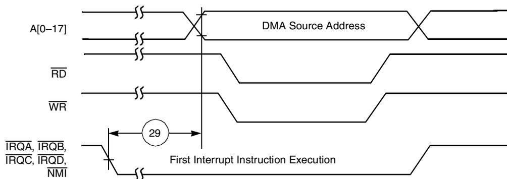
**Figure 2-11.** External Memory Access (DMA Source) Timing
