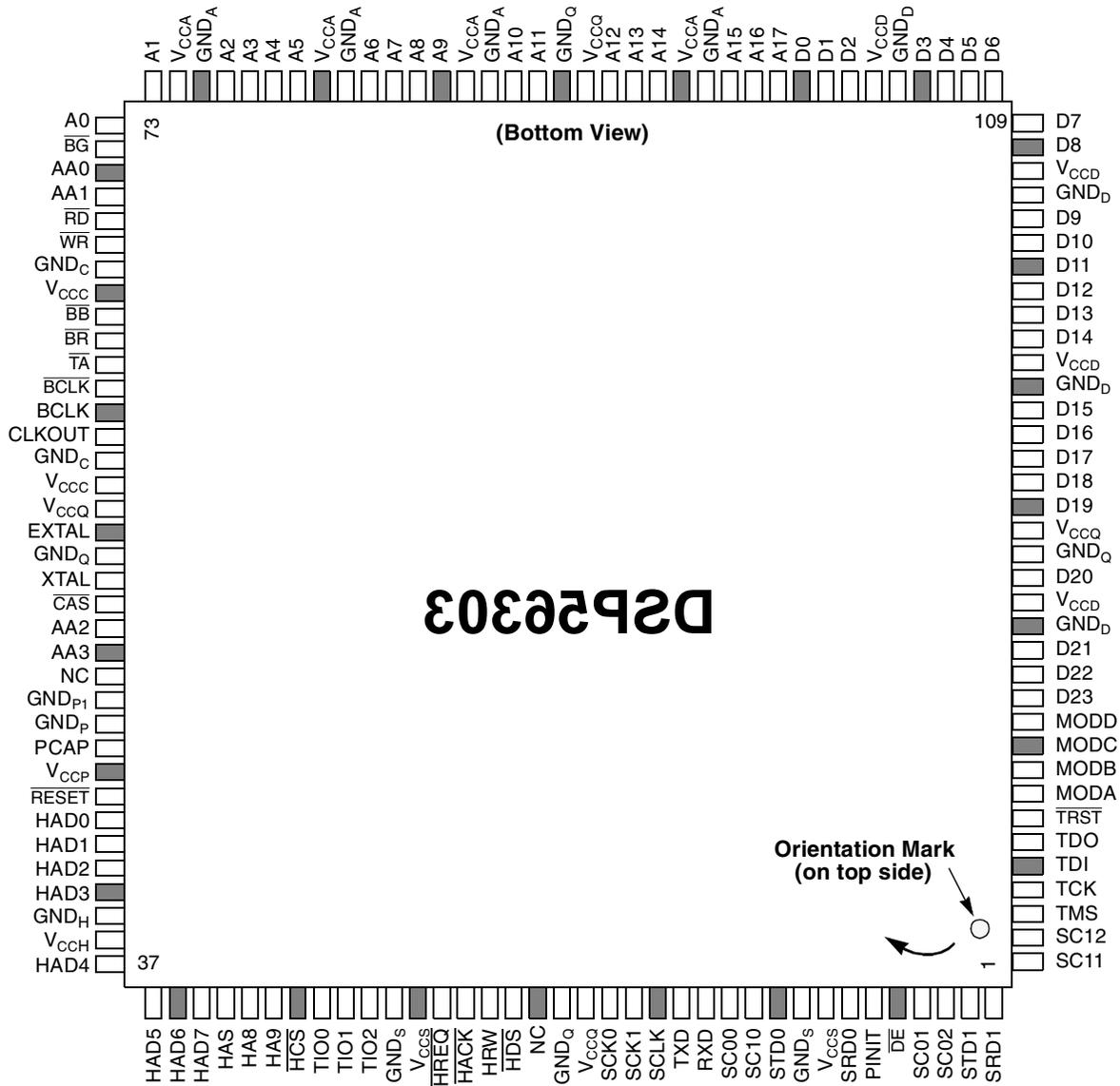
**Notes:** Because of size constraints in this figure, only one name is shown for multiplexed pins. Refer to **Table 3-1** and **Table 3-2** for detailed information about pin functions and signal names.
