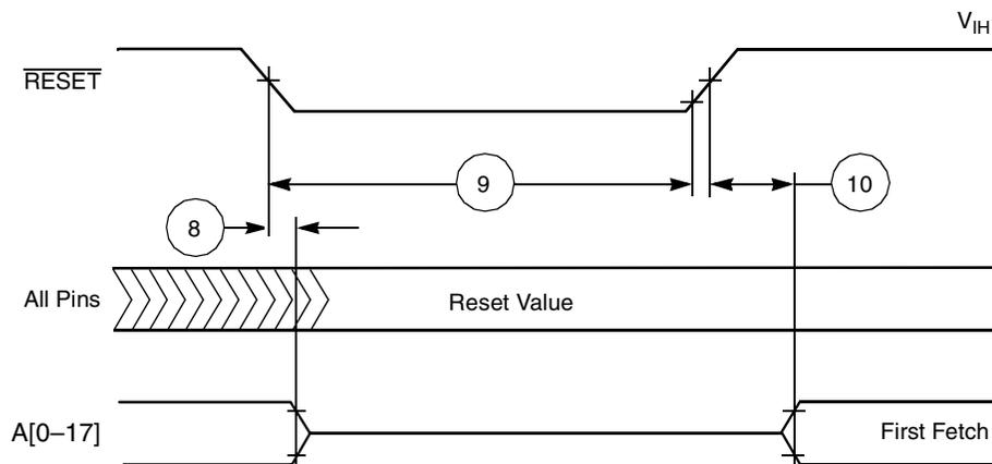
**Figure 2-3.** Reset Timing
