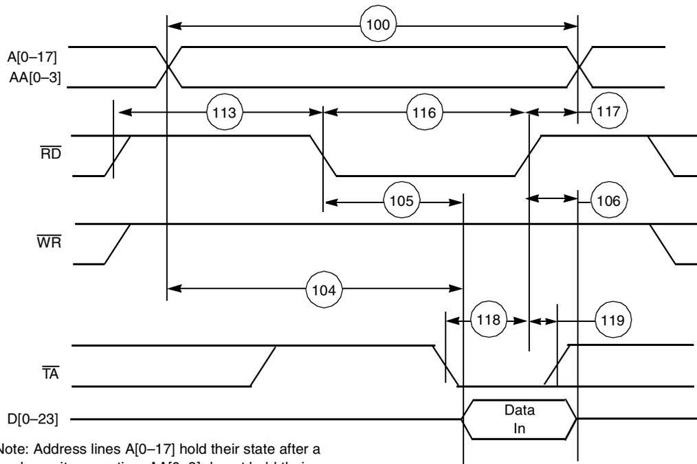
Note: Address lines A[0-17] hold their state after a read or write operation. AA[0-3] do not hold their state after a read or write operation.
