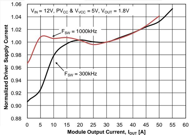
Figure 13. Driver Supply Current vs. Output Current
