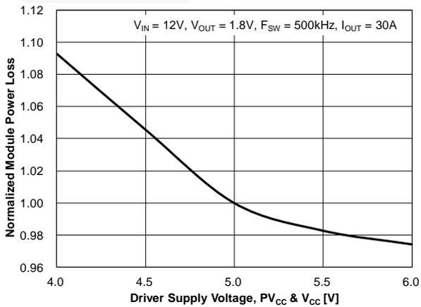
Figure 8. Power Loss vs. Driver Supply Voltage
