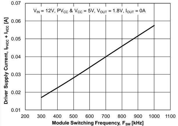
Figure 11. Driver Supply Current vs. Switching Frequency
