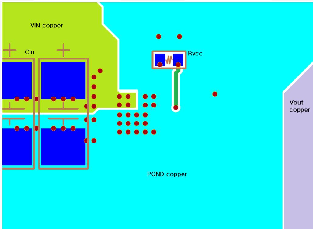
**Figure 40. Single-Phase Board Layout Example – Bottom View (Mirrored)**
