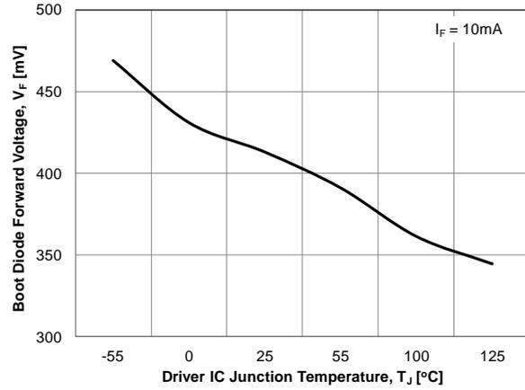
Figure 23. Boot Diode Forward Voltage vs. Temperature
