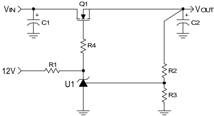
Figure 4 - Low cost 3.3V to 2.7V output.
