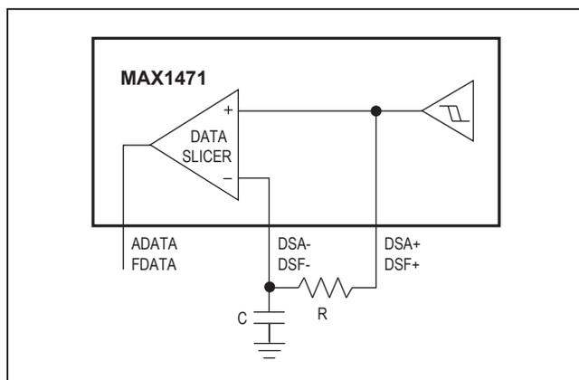
Figure 4. Generating Data-Slicer Threshold Using a Lowpass Filter
