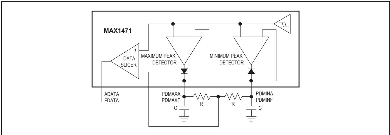
Figure 5. Generating Data-Slicer Threshold Using the Peak Detectors
