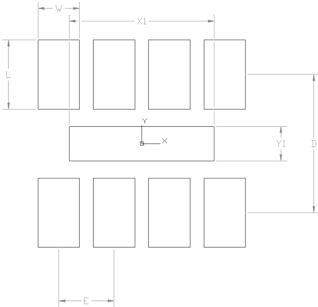
**Figure 8.1. Si51211 8-pin TDFN PCB Land Pattern**
