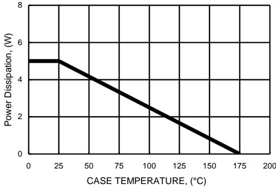
**FIG.2- Load Dump Power Characteristics**
