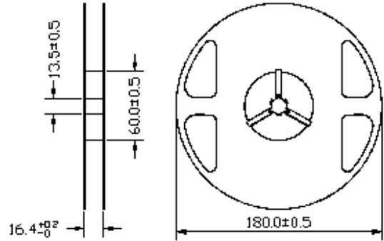
Dimensions of Tape (Unit: mm)
