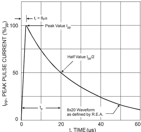
Fig. 3 Pulse Waveform
