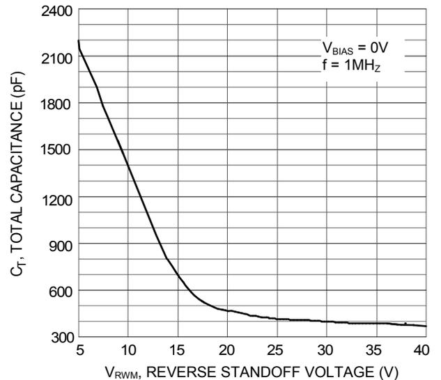
Fig. 6 Total Capacitance vs. Reverse Standoff Voltage
