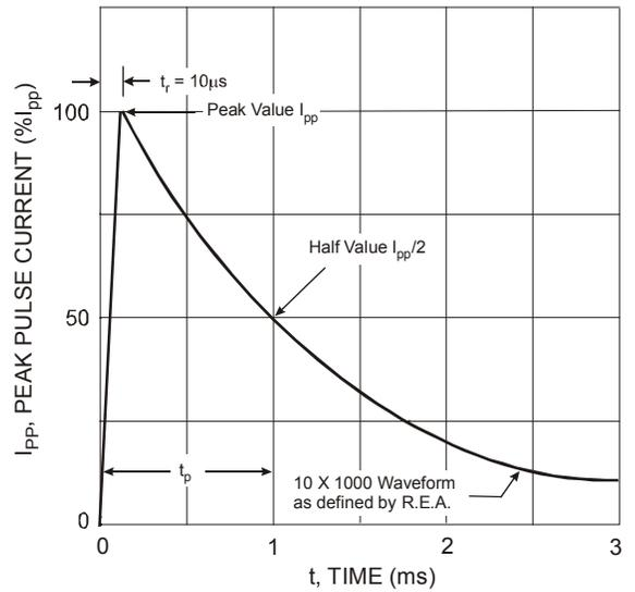
Fig. 2 Pulse Waveform
