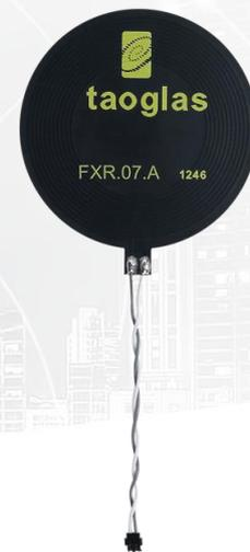
The FXR.07.52.0075X.A is a circular, flexible, NFC (Near Field Communications) antenna for use in mobile devices and other applications such as keycards, payment systems, and boarding passes. The design provides a flexible NFC antenna with 75mm twisted pair 28AWG cable that can be adhered to the plastic enclosure of the device for ease of installation and work with specific 13.56MHz RFID and NFC chips which need to connect via JST ACH connector.
