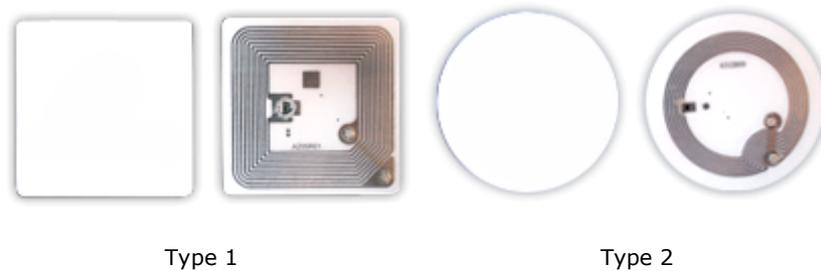
Type 1 tag is based on ISO/IEC 14443A standard and has 512 bytes of memory.
