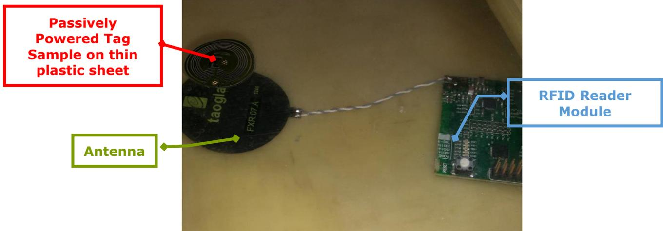
The test sample is placed on a thin sheet of plastic connected to the movable part of the fixture. Then the distance is carefully adjusted until the reader can no longer read the sample, thus the maximum interrogation distance is displayed in the ruler.
