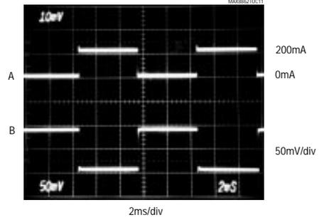
$V_{IN2} = 7V$ ,  $V_{OUT2} = 3.2V$
