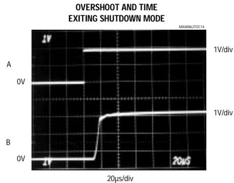
$V_{IN1} = 5.3V$ ,  $I_{OUT1} = 5mA$
