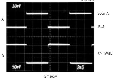
$V_{IN1} = 7V$ ,  $V_{OUT1} = 3.2V$
