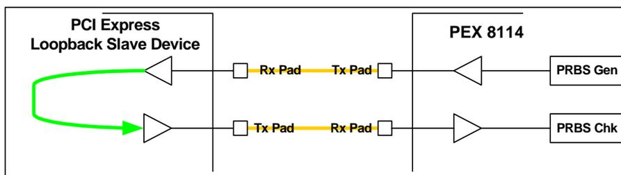
Figure 15-3. Cable Loopback
