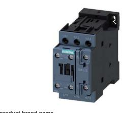
power contactor, AC-3 12 A, 5.5 kW / 400 V 1 NO + 1 NC, 24 V DC with integrated varistor 3-pole, size S0 screw terminal suitable for PLC outputs upright mounting position not expandable with auxiliary switch
