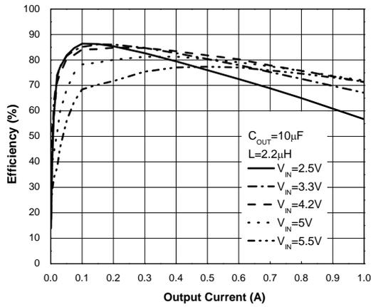
**Efficiency vs. Output Current ( $V_{OUT}=2.5V$ )**
