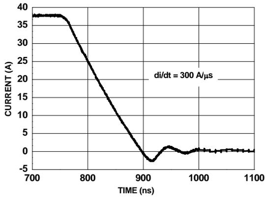
Figure 14. FDMS8558SDC SyncFET<sup>™</sup> body diode reverse recovery characteristic
