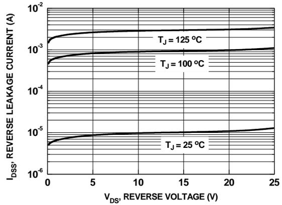
Figure 15. SyncFET<sup>™</sup> body diode reverse leakage versus drain-source voltage
