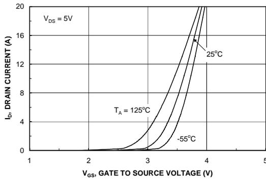
Figure 5. Transfer Characteristics.
