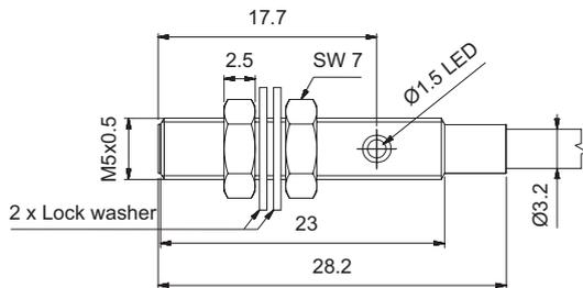
Fig. 13 Short body, flush version, cable
