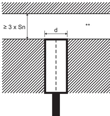
**Fig. 15** Flush sensor, when installed in damping material
