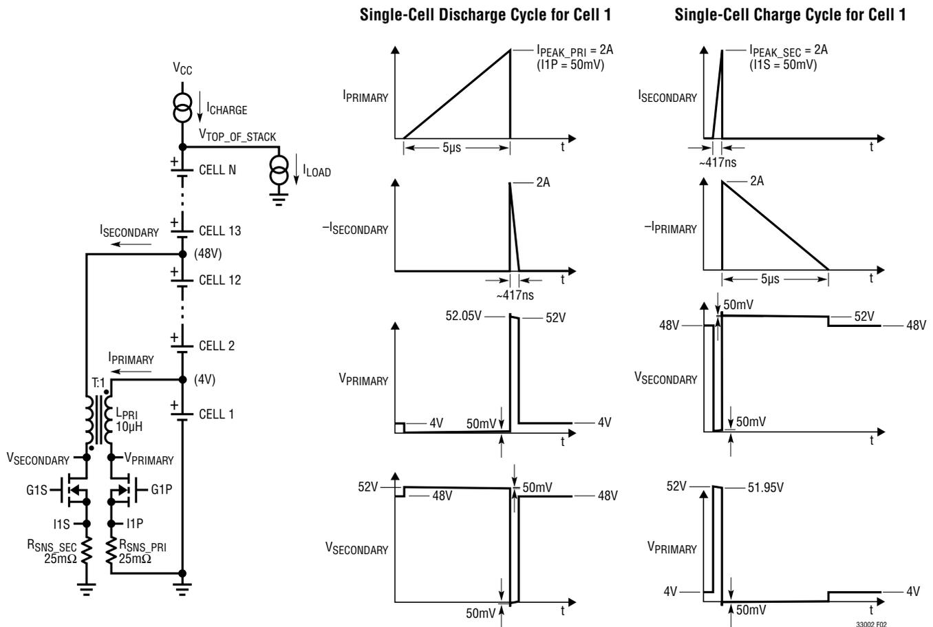
Figure 2. Synchronous Flyback Balancing Example with T = 1, S = 12
