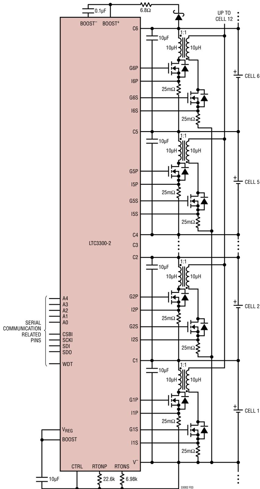
Figure 3. LTC3300-2 6-Cell Active Balancer Module Showing Power Connections for the Multi-Transformer Application (CTRL = V<sup>-</sup>)
