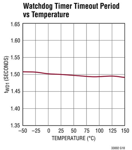
**TYPICAL PERFORMANCE CHARACTERISTICS**  $T_A = 25^\circ\text{C}$  unless otherwise specified.
