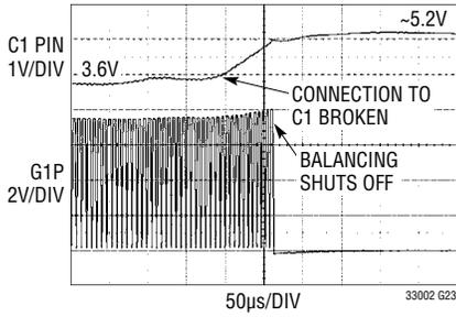
**Protection for Broken Connection to Secondary Stack While Discharging**
