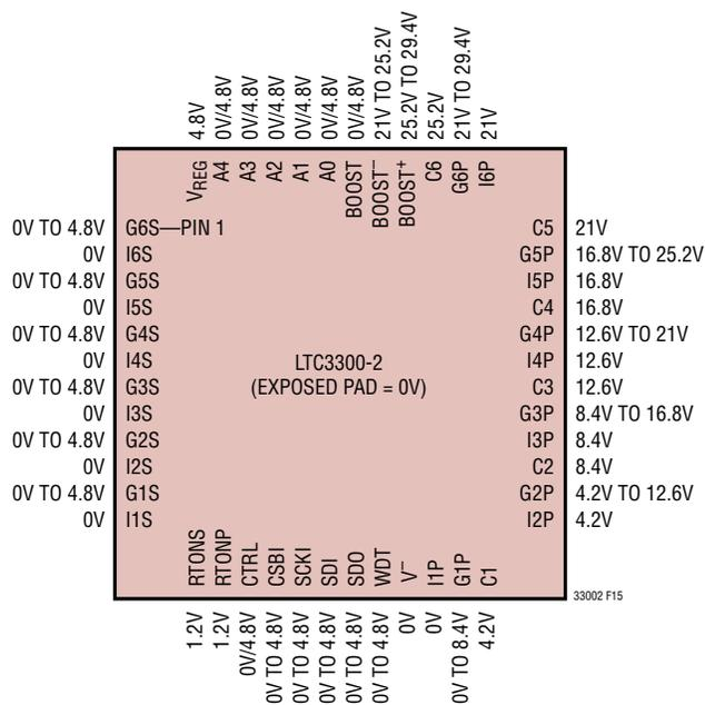
Figure 15. Typical Pin Voltages for Six 4.2V Cells
