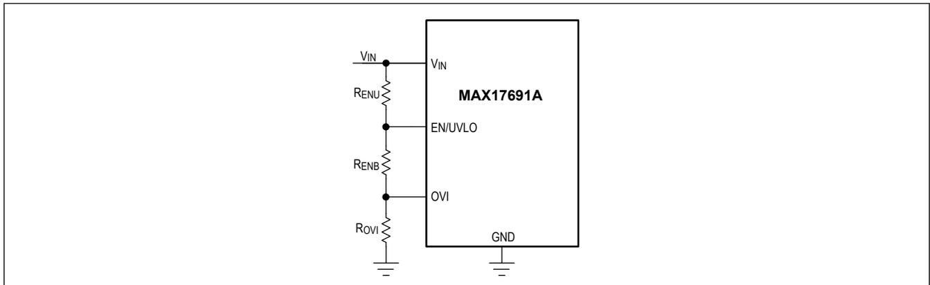
Figure 3. Programming EN/UVLO and OVI in MAX17691A
