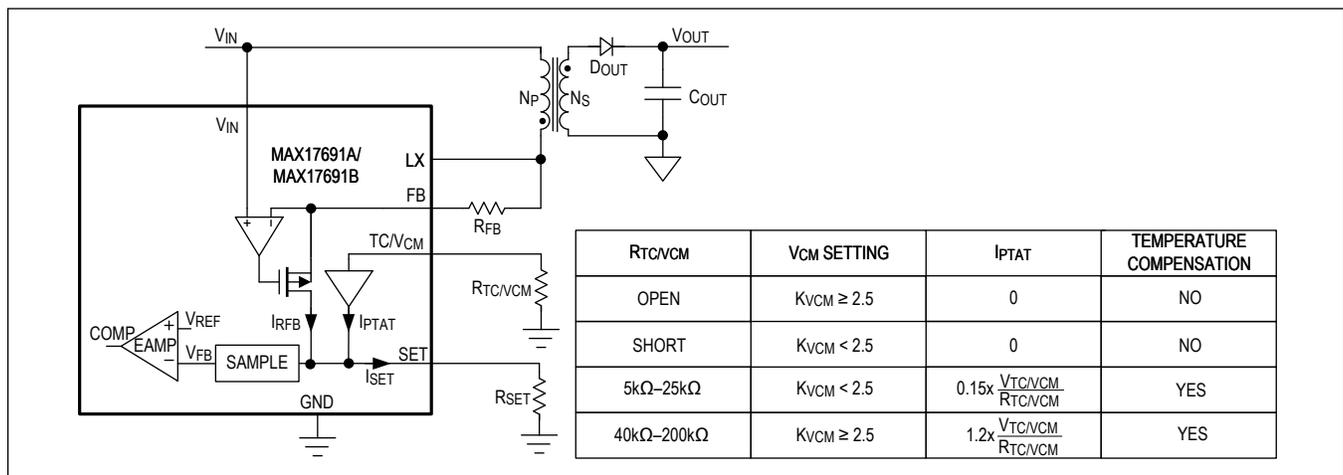
Figure 7. TC/V<sub>CM</sub> Pin Configuration
