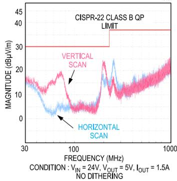
MAX17691A, 5V OUTPUT, 1.5A LOAD CURRENT
