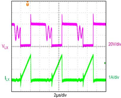
MAX17691B, STEADY-STATE SWITCHING WAVEFORMS
