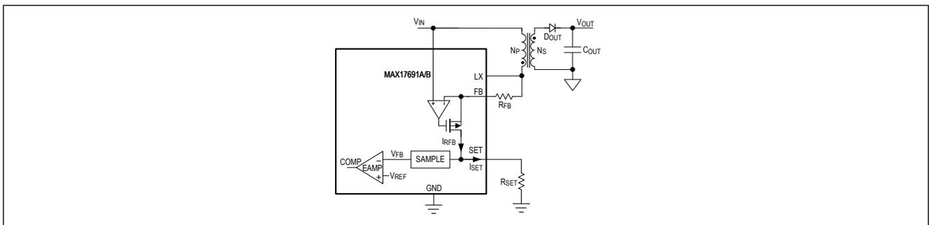
Figure 6. Simplified Diagram of No-Opto Flyback Operation
