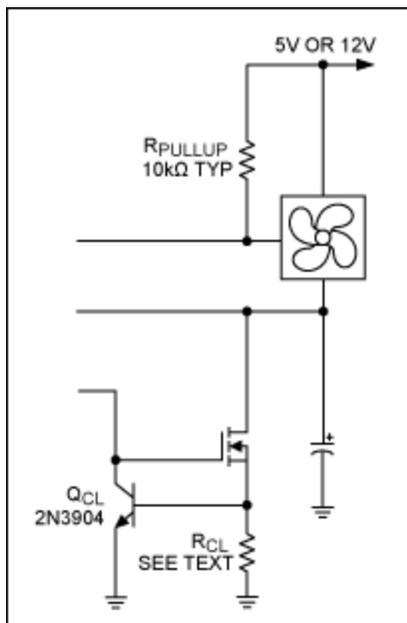
Figure 2. When current limiting is necessary for pass transistors, this circuit provides that function.
