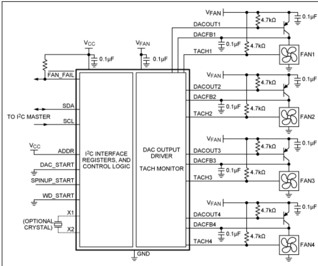
Figure 3. The MAX6620 shown here is a 4-channel linear fan-speed controller using external pass transistors to supply variable power to the fan. The MAX6620 monitors tachometer signals from the fans and adjusts the power-supply voltage so that the desired tachometer frequency is achieved.
