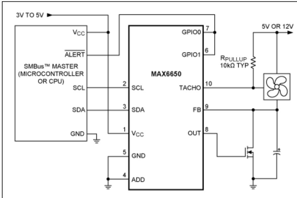
Figure 1. The MAX6650 is a true fan-speed regulator because it includes a tachometer output fan in its feedback loop.
