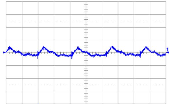
Fig. 2.0V.6: Output voltage ripple (20 mV/div.) at full rated load current into a resistive load with external capacitance  $47 \mu\text{F}$  ceramic +  $1 \mu\text{F}$  ceramic, and  $V_{in} = 12$  V for  $V_{out} = 2.0$  V. Time scale: 1  $\mu\text{s}$ /div.
