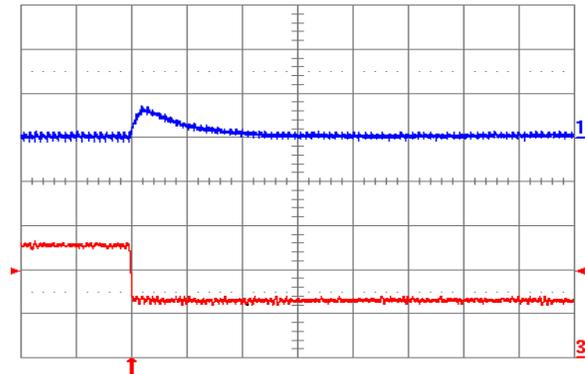
Fig. 1.5V.8: Output voltage response for  $V_{out} = 1.5\text{ V}$  to negative load current step change from 5 A to 2.5 A with slew rate of  $-5\text{ A}/\mu\text{s}$  at  $V_{in} = 12\text{ V}$ . Top trace: output voltage (100 mV/div.); Bottom trace: load current (2 A/div.).  $C_o = 47\text{ }\mu\text{F}$  ceramic. Time scale:  $20\text{ }\mu\text{s}/\text{div}$ .
