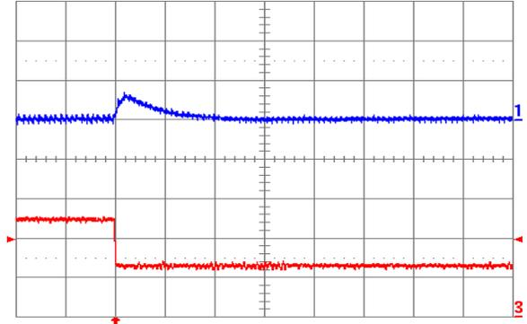
Fig. 2.0V.8: Output voltage response for  $V_{out} = 2.0\text{ V}$  to negative load current step change from 5 A to 2.5 A with slew rate of  $-5\text{ A}/\mu\text{s}$  at  $V_{in} = 12\text{ V}$ . Top trace: output voltage (100 mV/div.); Bottom trace: load current (2 A/div.).  $C_o = 47\text{ }\mu\text{F}$  ceramic. Time scale:  $20\text{ }\mu\text{s}/\text{div}$ .
