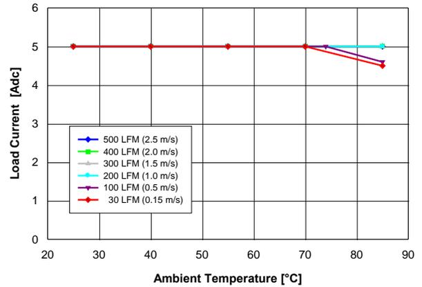
Fig. 5.0V.2: Available load current vs. ambient temperature and airflow rates for  $V_{out} = 5.0$  V converter mounted horizontally with  $V_{in} = 12$  V, and maximum MOSFET temperature  $\leq 120$  °C.
