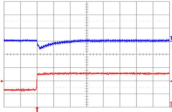
Fig. 1.5V.7: Output voltage response for  $V_{out} = 1.5\text{ V}$  to positive load current step change from 2.5 A to 5 A with slew rate of  $5\text{ A}/\mu\text{s}$  at  $V_{in} = 12\text{ V}$ . Top trace: output voltage (100 mV/div.); Bottom trace: load current (2 A/div.).  $C_o = 47\text{ }\mu\text{F}$  ceramic. Time scale:  $20\text{ }\mu\text{s}/\text{div}$ .
