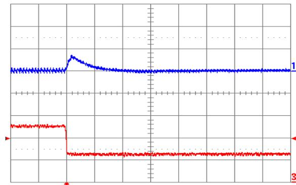
Fig. 2.5V.8: Output voltage response for  $V_{out} = 2.5\text{ V}$  to negative load current step change from 5 A to 2.5 A with slew rate of  $-5\text{ A}/\mu\text{s}$  at  $V_{in} = 12\text{ V}$ . Top trace: output voltage (100 mV/div.); Bottom trace: load current (2 A/div.).  $C_o = 47\text{ }\mu\text{F}$  ceramic. Time scale: 20  $\mu\text{s}$ /div.
