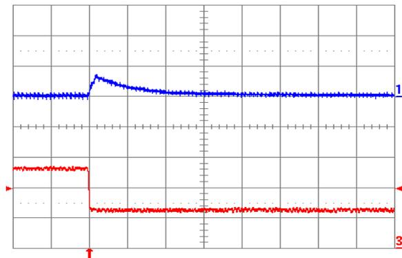
Fig. 1.0V.8: Output voltage response for  $V_{out} = 1.0$  V to negative load current step change from 5 A to 2.5 A with slew rate of  $-5 \text{ A}/\mu\text{s}$  at  $V_{in} = 12$  V. Top trace: output voltage (100 mV/div.); Bottom trace: load current (2 A/div.).  $C_o = 47 \mu\text{F}$  ceramic. Time scale: 20  $\mu\text{s}$ /div.
