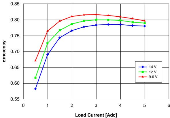
Fig. 1.2V.3: Efficiency vs. load current and input voltage for  $V_{out} = 1.2\text{ V}$  converter mounted vertically with air flowing at a rate of 200 LFM (1 m/s) and  $T_a = 25\text{ }^{\circ}\text{C}$ .
