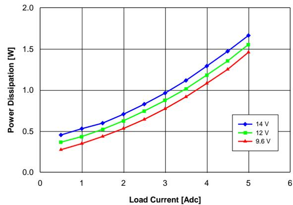
Fig. 1.0V.4: Power Loss vs. load current and input voltage for  $V_{out} = 1.0\text{ V}$  converter mounted vertically with air flowing at a rate of  $200\text{ LFM}$  ( $1\text{ m/s}$ ) and  $T_a = 25\text{ }^\circ\text{C}$ .
