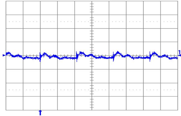
Fig. 1.0V.6: Output voltage ripple (20 mV/div.) at full rated load current into a resistive load with external capacitance  $47 \mu\text{F}$  ceramic +  $1 \mu\text{F}$  ceramic, and  $V_{in} = 12$  V for  $V_{out} = 1.0$  V. Time scale: 1  $\mu\text{s}$ /div.
