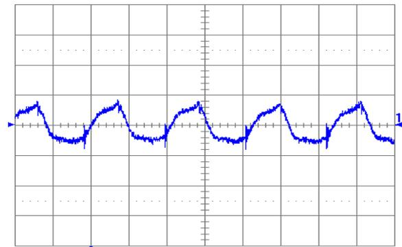
Fig. 5.0V.6: Output voltage ripple (20 mV/div.) at full rated load current into a resistive load with external capacitance  $47 \mu\text{F}$  ceramic +  $1 \mu\text{F}$  ceramic, and  $V_{in} = 12$  V for  $V_{out} = 5.0$  V. Time scale: 1  $\mu\text{s}$ /div.
