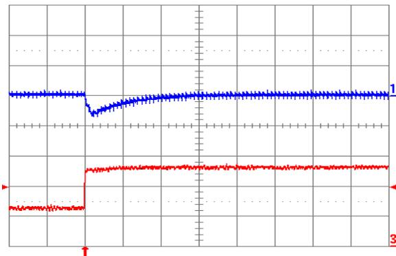
Fig. 1.0V.7: Output voltage response for  $V_{out} = 1.0$  V to positive load current step change from 2.5 A to 5 A with slew rate of  $5 \text{ A}/\mu\text{s}$  at  $V_{in} = 12$  V. Top trace: output voltage (100 mV/div.); Bottom trace: load current (2 A/div.).  $C_o = 47 \mu\text{F}$  ceramic. Time scale: 20  $\mu\text{s}$ /div.
