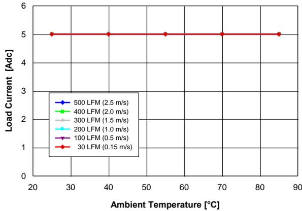
Fig. 1.2V.1: Available load current vs. ambient temperature and airflow rates for  $V_{out} = 1.2\text{ V}$  converter mounted vertically with  $V_{in} = 12\text{ V}$ , and maximum MOSFET temperature  $\leq 120\text{ }^{\circ}\text{C}$ .
