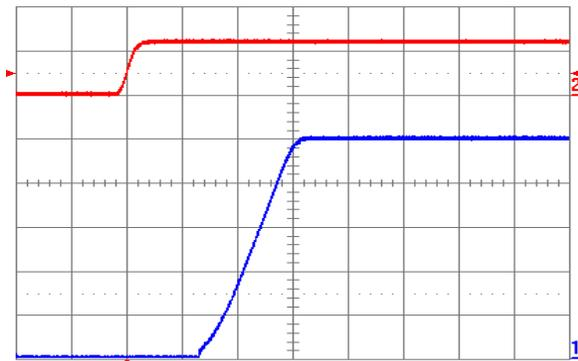
Fig. 5.0V.5: Turn-on transient for  $V_{out} = 5.0$  V with application of  $V_{in}$  at full rated load current (resistive) and  $47 \mu\text{F}$  external capacitance at  $V_{in} = 12$  V. Top trace:  $V_{in}$  (10 V/div.); Bottom trace: output voltage (1 V/div.); Time scale: 5 ms/div.
