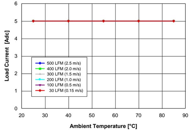
Fig. 2.0V.2: Available load current vs. ambient temperature and airflow rates for  $V_{out} = 2.0$  V converter mounted horizontally with  $V_{in} = 12$  V, and maximum MOSFET temperature  $\leq 120$  °C.
