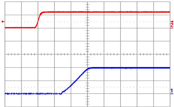
Fig. 2.0V.5: Turn-on transient for  $V_{out} = 2.0$  V with application of  $V_{in}$  at full rated load current (resistive) and  $47 \mu\text{F}$  external capacitance at  $V_{in} = 12$  V. Top trace:  $V_{in}$  (10 V/div.); Bottom trace: output voltage (1 V/div.); Time scale: 5 ms/div.
