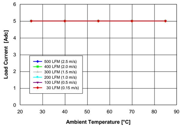
Fig. 1.8V.2: Available load current vs. ambient temperature and airflow rates for  $V_{out} = 1.8\text{ V}$  converter mounted horizontally with  $V_{in} = 12\text{ V}$ , and maximum MOSFET temperature  $\leq 120\text{ }^\circ\text{C}$ .
