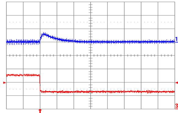
Fig. 1.8V.8: Output voltage response for  $V_{out} = 1.8\text{ V}$  to negative load current step change from 5 A to 2.5 A with slew rate of  $-5\text{ A}/\mu\text{s}$  at  $V_{in} = 12\text{ V}$ . Top trace: output voltage (100 mV/div.); Bottom trace: load current (2 A/div.).  $C_o = 47\text{ }\mu\text{F}$  ceramic. Time scale: 20  $\mu\text{s}$ /div.
