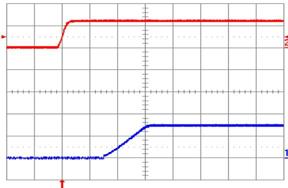
Fig. 1.5V.5: Turn-on transient for  $V_{out} = 1.5\text{ V}$  with application of  $V_{in}$  at full rated load current (resistive) and  $47\text{ }\mu\text{F}$  external capacitance at  $V_{in} = 12\text{ V}$ . Top trace:  $V_{in}$  (10 V/div.); Bottom trace: output voltage (1 V/div.); Time scale: 5 ms/div.
