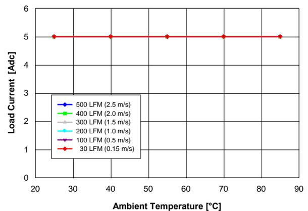
Fig. 2.5V.2: Available load current vs. ambient temperature and airflow rates for  $V_{out} = 2.5\text{ V}$  converter mounted horizontally with  $V_{in} = 12\text{ V}$ , and maximum MOSFET temperature  $\leq 120\text{ }^\circ\text{C}$ .
