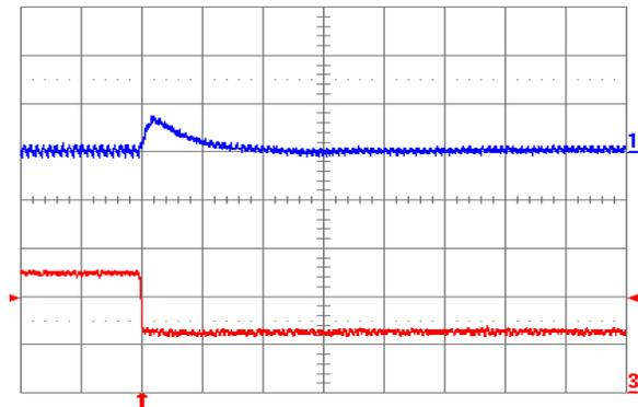
Fig. 3.3V.8: Output voltage response for  $V_{out} = 3.3\text{ V}$  to negative load current step change from 5 A to 2.5 A with slew rate of  $-5\text{ A}/\mu\text{s}$  at  $V_{in} = 12\text{ V}$ . Top trace: output voltage (100 mV/div.); Bottom trace: load current (2 A/div.).  $C_o = 47\ \mu\text{F}$  ceramic. Time scale: 20  $\mu\text{s}$ /div.
