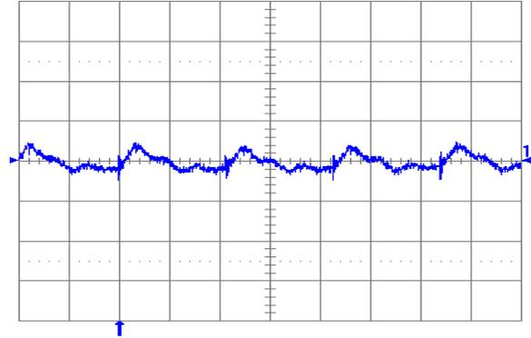
Fig. 1.8V.6: Output voltage ripple (20 mV/div.) at full rated load current into a resistive load with external capacitance  $47\text{ }\mu\text{F}$  ceramic +  $1\text{ }\mu\text{F}$  ceramic, and  $V_{in} = 12\text{ V}$  for  $V_{out} = 1.8\text{ V}$ . Time scale: 1  $\mu\text{s}$ /div.
