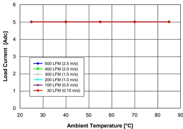
Fig. 1.5V.1: Available load current vs. ambient temperature and airflow rates for  $V_{out} = 1.5\text{ V}$  converter mounted vertically with  $V_{in} = 12\text{ V}$ , and maximum MOSFET temperature  $\leq 120\text{ }^\circ\text{C}$ .
