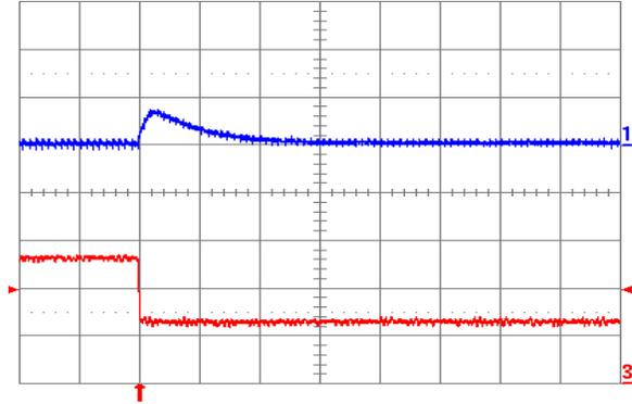
Fig. 1.2V.8: Output voltage response for  $V_{out} = 1.2\text{ V}$  to negative load current step change from  $5\text{ A}$  to  $2.5\text{ A}$  with slew rate of  $-5\text{ A}/\mu\text{s}$  at  $V_{in} = 12\text{ V}$ . Top trace: output voltage ( $100\text{ mV}/\text{div.}$ ); Bottom trace: load current ( $2\text{ A}/\text{div.}$ ).  $C_o = 47\text{ }\mu\text{F}$  ceramic. Time scale:  $20\text{ }\mu\text{s}/\text{div.}$
