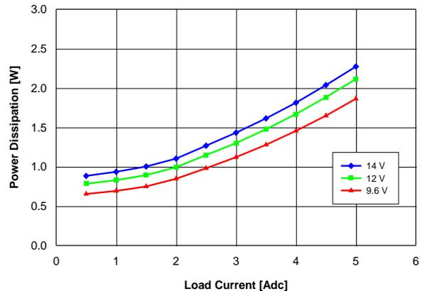
Fig. 3.3V.4: Power Loss vs. load current and input voltage for  $V_{out} = 3.3\text{ V}$  converter mounted vertically with air flowing at a rate of  $200\text{ LFM}$  ( $1\text{ m/s}$ ) and  $T_a = 25\text{ }^\circ\text{C}$ .
