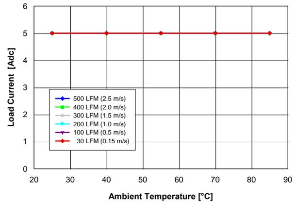
Fig. 1.0V.2: Available load current vs. ambient temperature and airflow rates for  $V_{out} = 1.0\text{ V}$  converter mounted horizontally with  $V_{in} = 12\text{ V}$ , and maximum MOSFET temperature  $\leq 120\text{ }^\circ\text{C}$ .
