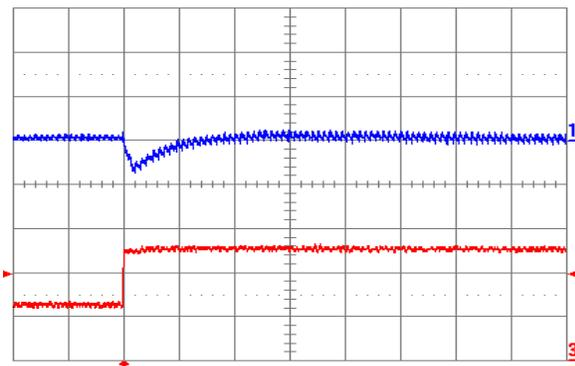
Fig. 2.5V.7: Output voltage response for  $V_{out} = 2.5\text{ V}$  to positive load current step change from 2.5 A to 5 A with slew rate of  $5\text{ A}/\mu\text{s}$  at  $V_{in} = 12\text{ V}$ . Top trace: output voltage (100 mV/div.); Bottom trace: load current (2 A/div.).  $C_o = 47\text{ }\mu\text{F}$  ceramic. Time scale: 20  $\mu\text{s}$ /div.
