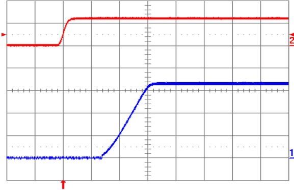
Fig. 3.3V.5: Turn-on transient for  $V_{out} = 3.3\text{ V}$  with application of  $V_{in}$  at full rated load current (resistive) and  $47\ \mu\text{F}$  external capacitance at  $V_{in} = 12\text{ V}$ . Top trace:  $V_{in}$  (10 V/div.); Bottom trace: output voltage (1 V/div.); Time scale: 5 ms/div.
