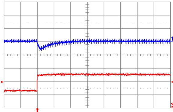
Fig. 1.8V.7: Output voltage response for  $V_{out} = 1.8\text{ V}$  to positive load current step change from 2.5 A to 5 A with slew rate of  $5\text{ A}/\mu\text{s}$  at  $V_{in} = 12\text{ V}$ . Top trace: output voltage (100 mV/div.); Bottom trace: load current (2 A/div.).  $C_o = 47\text{ }\mu\text{F}$  ceramic. Time scale: 20  $\mu\text{s}$ /div.
