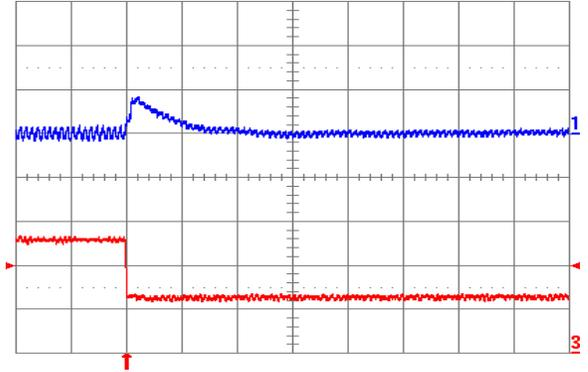
Fig. 5.0V.8: Output voltage response for  $V_{out} = 5.0\text{ V}$  to negative load current step change from  $5\text{ A}$  to  $2.5\text{ A}$  with slew rate of  $-5\text{ A}/\mu\text{s}$  at  $V_{in} = 12\text{ V}$ . Top trace: output voltage ( $100\text{ mV}/\text{div.}$ ); Bottom trace: load current ( $2\text{ A}/\text{div.}$ ).  $C_o = 47\text{ }\mu\text{F}$  ceramic. Time scale:  $20\text{ }\mu\text{s}/\text{div.}$
