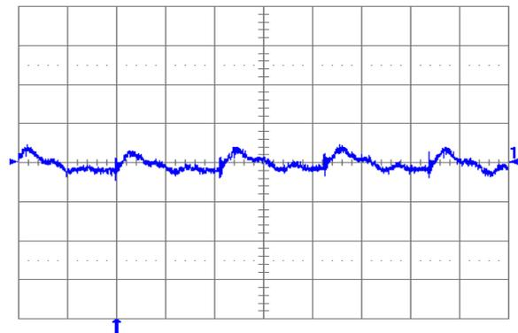
Fig. 1.5V.6: Output voltage ripple (20 mV/div.) at full rated load current into a resistive load with external capacitance  $47\text{ }\mu\text{F}$  ceramic +  $1\text{ }\mu\text{F}$  ceramic, and  $V_{in} = 12\text{ V}$  for  $V_{out} = 1.5\text{ V}$ . Time scale:  $1\text{ }\mu\text{s}/\text{div}$ .
