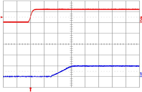
Fig. 1.0V.5: Turn-on transient for  $V_{out} = 1.0$  V with application of  $V_{in}$  at full rated load current (resistive) and  $47 \mu\text{F}$  external capacitance at  $V_{in} = 12$  V. Top trace:  $V_{in}$  (10 V/div.); Bottom trace: output voltage (1 V/div.); Time scale: 5 ms/div.
