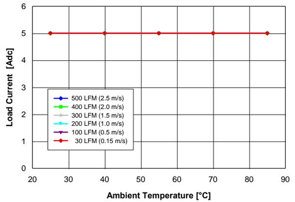
Fig. 3.3V.2: Available load current vs. ambient temperature and airflow rates for  $V_{out} = 3.3\text{ V}$  converter mounted horizontally with  $V_{in} = 12\text{ V}$ , and maximum MOSFET temperature  $\leq 120\text{ }^\circ\text{C}$ .
