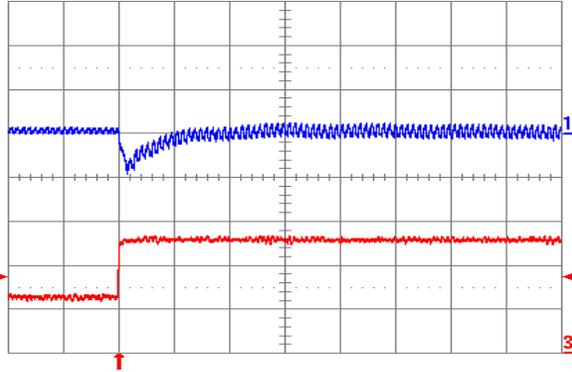
Fig. 5.0V.7: Output voltage response for  $V_{out} = 5.0\text{ V}$  to positive load current step change from  $2.5\text{ A}$  to  $5\text{ A}$  with slew rate of  $5\text{ A}/\mu\text{s}$  at  $V_{in} = 12\text{ V}$ . Top trace: output voltage ( $100\text{ mV}/\text{div.}$ ); Bottom trace: load current ( $2\text{ A}/\text{div.}$ ).  $C_o = 47\text{ }\mu\text{F}$  ceramic. Time scale:  $20\text{ }\mu\text{s}/\text{div.}$
