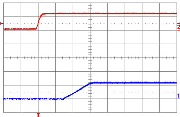
Fig. 1.2V.5: Turn-on transient for  $V_{out} = 1.2\text{ V}$  with application of  $V_{in}$  at full rated load current (resistive) and  $47\text{ }\mu\text{F}$  external capacitance at  $V_{in} = 12\text{ V}$ . Top trace:  $V_{in}$  (10 V/div.); Bottom trace: output voltage (1 V/div.); Time scale: 5 ms/div.
