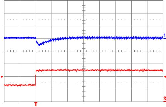
Fig. 2.0V.7: Output voltage response for  $V_{out} = 2.0\text{ V}$  to positive load current step change from 2.5 A to 5 A with slew rate of  $5\text{ A}/\mu\text{s}$  at  $V_{in} = 12\text{ V}$ . Top trace: output voltage (100 mV/div.); Bottom trace: load current (2 A/div.).  $C_o = 47\text{ }\mu\text{F}$  ceramic. Time scale:  $20\text{ }\mu\text{s}/\text{div}$ .
