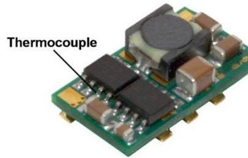
Fig. C. Location of the thermocouple for thermal testing.
