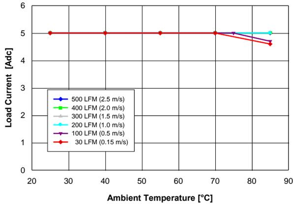
Fig. 5.0V.1: Available load current vs. ambient temperature and airflow rates for  $V_{out} = 5.0$  V converter mounted vertically with  $V_{in} = 12$  V, and maximum MOSFET temperature  $\leq 120$  °C.
