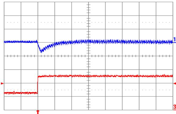
Fig. 3.3V.7: Output voltage response for  $V_{out} = 3.3\text{ V}$  to positive load current step change from 2.5 A to 5 A with slew rate of  $5\text{ A}/\mu\text{s}$  at  $V_{in} = 12\text{ V}$ . Top trace: output voltage (100 mV/div.); Bottom trace: load current (2 A/div.).  $C_o = 47\ \mu\text{F}$  ceramic. Time scale: 20  $\mu\text{s}$ /div.
