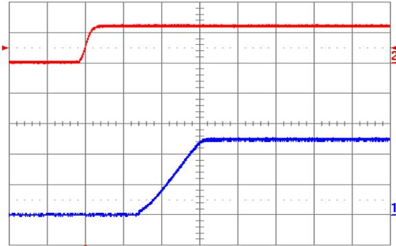
Fig. 2.5V.5: Turn-on transient for  $V_{out} = 2.5\text{ V}$  with application of  $V_{in}$  at full rated load current (resistive) and  $47\text{ }\mu\text{F}$  external capacitance at  $V_{in} = 12\text{ V}$ . Top trace:  $V_{in}$  (10 V/div.); Bottom trace: output voltage (1 V/div.); Time scale: 5 ms/div.
