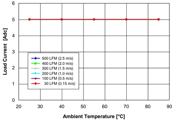
Fig. 2.0V.1: Available load current vs. ambient temperature and airflow rates for  $V_{out} = 2.0$  V converter mounted vertically with  $V_{in} = 12$  V, and maximum MOSFET temperature  $\leq 120$  °C.
