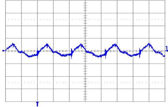
Fig. 3.3V.6: Output voltage ripple (20 mV/div.) at full rated load current into a resistive load with external capacitance  $47\ \mu\text{F}$  ceramic +  $1\ \mu\text{F}$  ceramic, and  $V_{in} = 12\text{ V}$  for  $V_{out} = 3.3\text{ V}$ . Time scale: 1  $\mu\text{s}$ /div.
