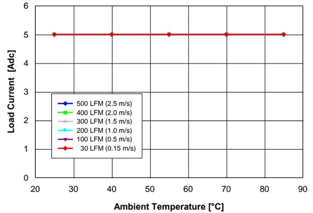
Fig. 1.2V.2: Available load current vs. ambient temperature and airflow rates for  $V_{out} = 1.2\text{ V}$  converter mounted horizontally with  $V_{in} = 12\text{ V}$ , and maximum MOSFET temperature  $\leq 120\text{ }^{\circ}\text{C}$ .
