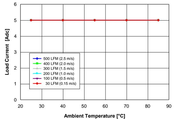
Fig. 1.5V.2: Available load current vs. ambient temperature and airflow rates for  $V_{out} = 1.5\text{ V}$  converter mounted horizontally with  $V_{in} = 12\text{ V}$ , and maximum MOSFET temperature  $\leq 120\text{ }^\circ\text{C}$ .
