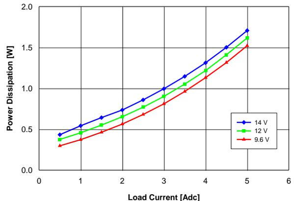
Fig. 1.2V.4: Power Loss vs. load current and input voltage for  $V_{out} = 1.2\text{ V}$  converter mounted vertically with air flowing at a rate of 200 LFM (1 m/s) and  $T_a = 25\text{ }^{\circ}\text{C}$ .
