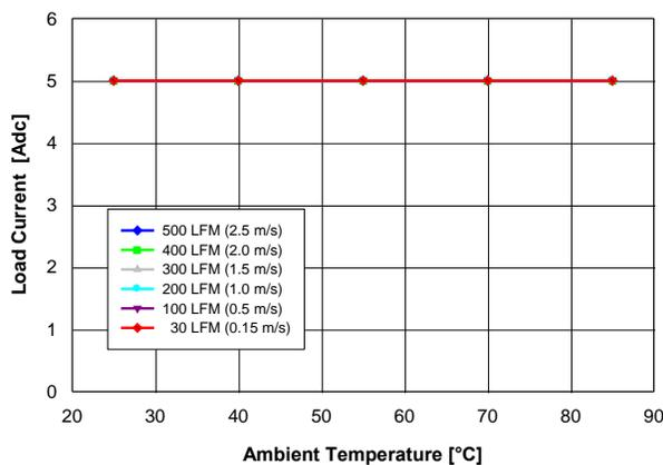
Fig. 2.5V.1: Available load current vs. ambient temperature and airflow rates for  $V_{out} = 2.5\text{ V}$  converter mounted vertically with  $V_{in} = 12\text{ V}$ , and maximum MOSFET temperature  $\leq 120\text{ }^\circ\text{C}$ .
