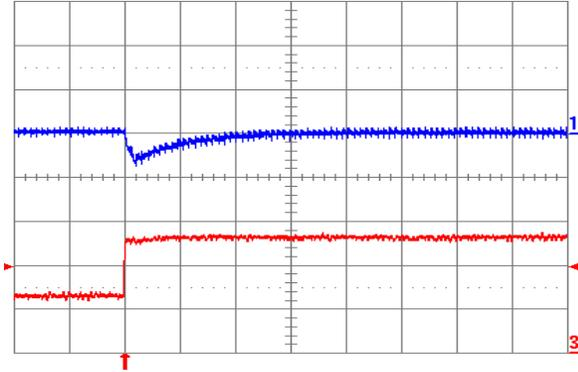
Fig. 1.2V.7: Output voltage response for  $V_{out} = 1.2\text{ V}$  to positive load current step change from  $2.5\text{ A}$  to  $5\text{ A}$  with slew rate of  $5\text{ A}/\mu\text{s}$  at  $V_{in} = 12\text{ V}$ . Top trace: output voltage ( $100\text{ mV}/\text{div.}$ ); Bottom trace: load current ( $2\text{ A}/\text{div.}$ ).  $C_o = 47\text{ }\mu\text{F}$  ceramic. Time scale:  $20\text{ }\mu\text{s}/\text{div.}$
