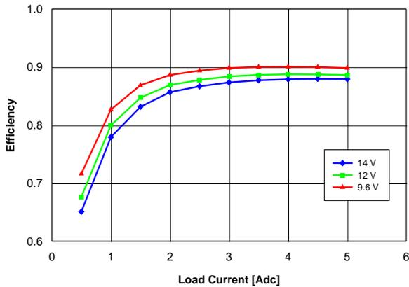
Fig. 3.3V.3: Efficiency vs. load current and input voltage for  $V_{out} = 3.3\text{ V}$  converter mounted vertically with air flowing at a rate of  $200\text{ LFM}$  ( $1\text{ m/s}$ ) and  $T_a = 25\text{ }^\circ\text{C}$ .
