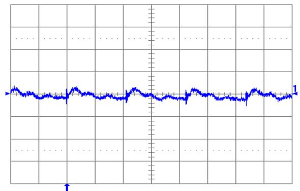
Fig. 1.2V.6: Output voltage ripple (20 mV/div.) at full rated load current into a resistive load with external capacitance  $47\text{ }\mu\text{F}$  ceramic +  $1\text{ }\mu\text{F}$  ceramic, and  $V_{in} = 12\text{ V}$  for  $V_{out} = 1.2\text{ V}$ . Time scale: 1  $\mu\text{s}$ /div.
