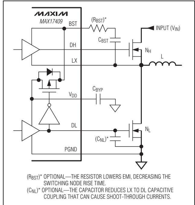
Figure 7. Gate-Drive Circuit
