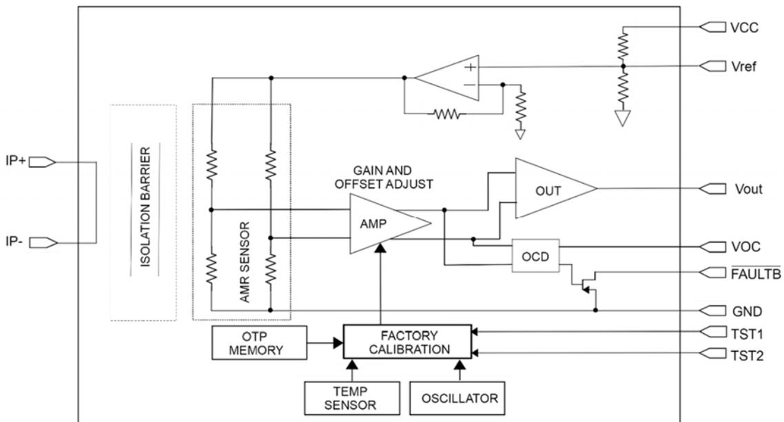
Figure 2 - Block diagram for fixed gain output products
