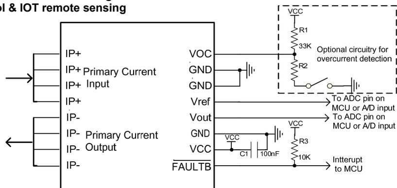
Figure 1 - Application circuit
