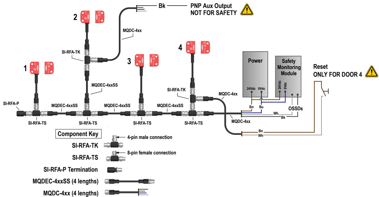
In long chains, or chains with a lot of ISD devices, the voltage at the first device (device closest to terminating plug) must stay above 19.5 V for the chain to operate properly.
