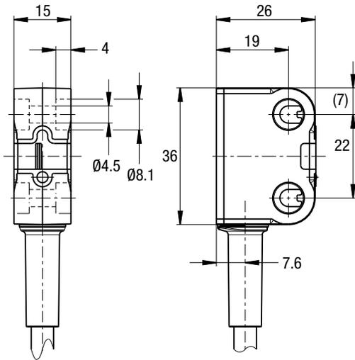
Figure 12. SI-RF Safety Switch Actuator
