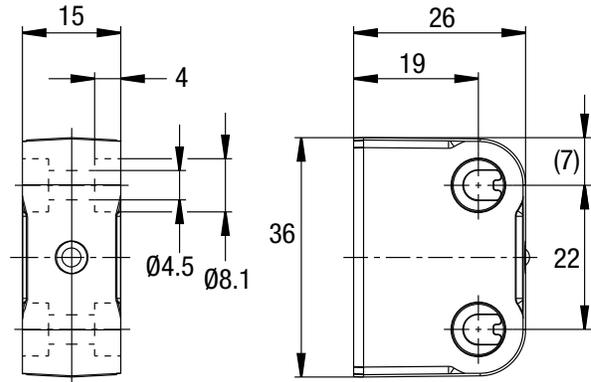
Figure 13. SI-RF Safety Switch -A2 Actuator
