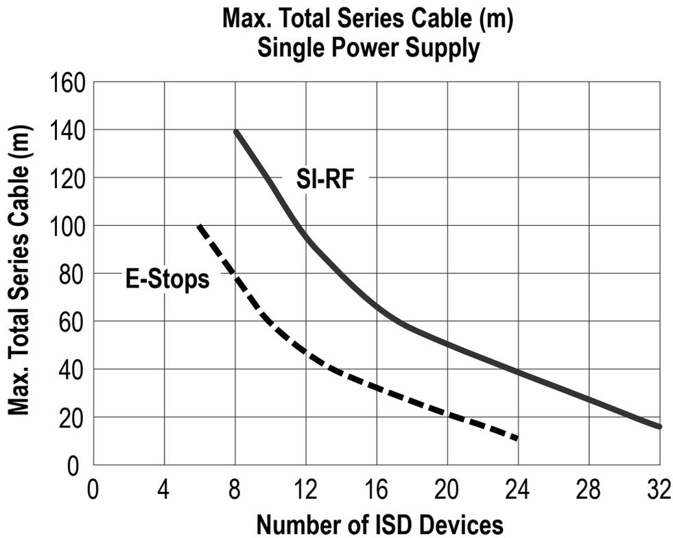
The SI-RFD switches and the ISD Connect have similar current demands. However, when used with a number of lighted ISD emergency stop devices, the current draw of the emergency stop devices governs the cable lengths and when more power is needed.
