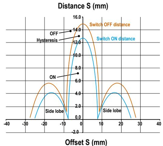
Figure 3. Sensor and actuator active areas
