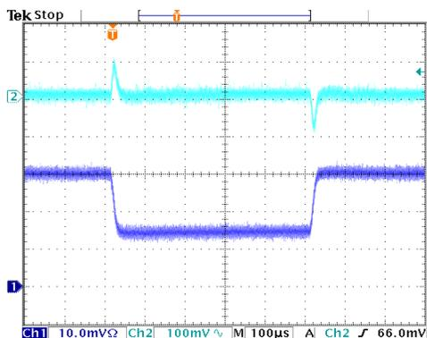
Fig. 14: Load Transient Response
