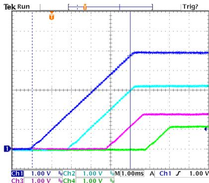
Fig. 10: Sequential Start-up Configuration
