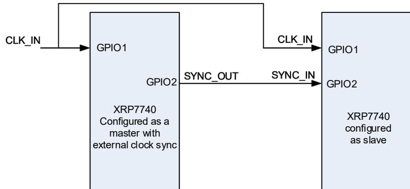
Fig. 25: External Clock Synchronization Master Slave Combination
