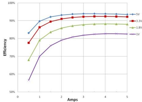
Fig. 4: 12Vin Efficiency: Single Channel 300kHz - Channels not in use are disabled
