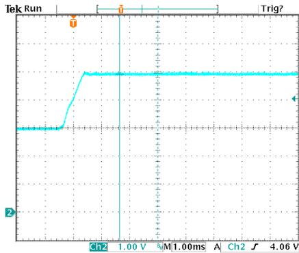
Fig. 12: Startup into 3V prebias – 5V Output
