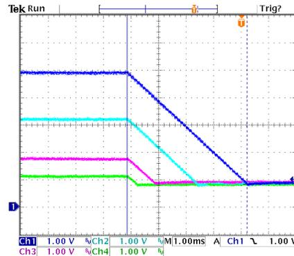
Fig. 13: Sequential Soft-Stop Configuration
