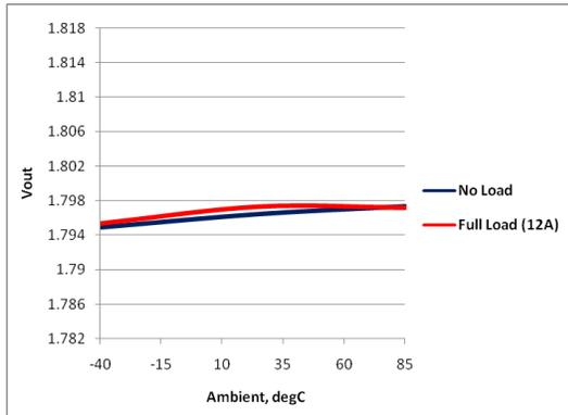
Fig. 15: XRP7740 Temperature Regulation
