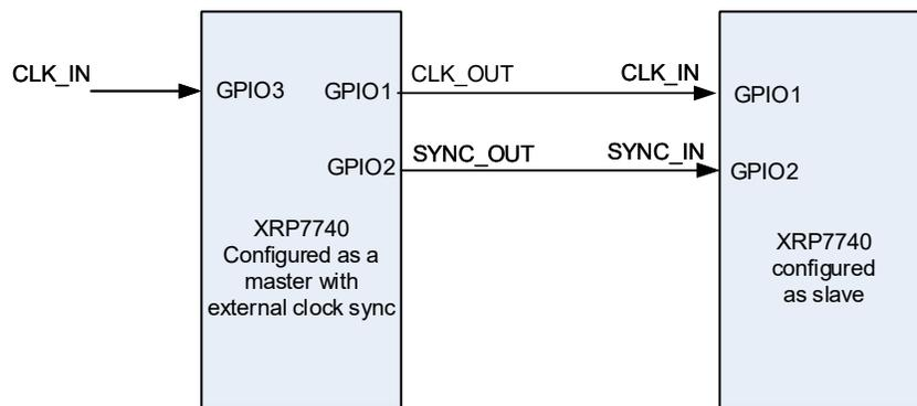
Fig. 26: Alternative External clock synchronization Master Slave combination
