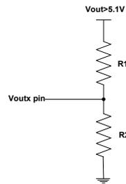
Fig.19: External divider network for high output voltage
