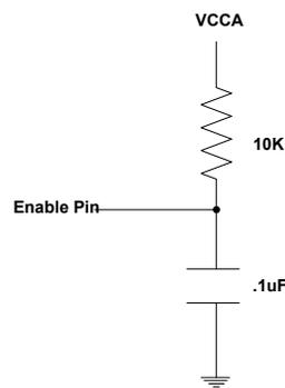
Fig. 17: RC Delay for Enable taken from VCCA
