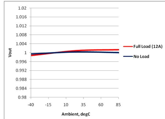
Fig. 16: XRP7740 Temperature Regulation
