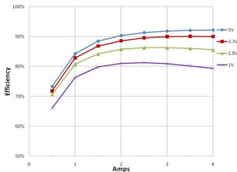
Fig. 6: 12Vin Efficiency: Single Channel 300kHz - Channels not in use are disabled
