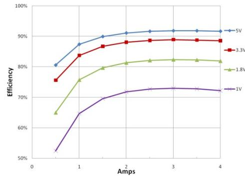
Fig. 7: 12Vin Efficiency: Single Channel 1MHz - Channels not in use are disabled
