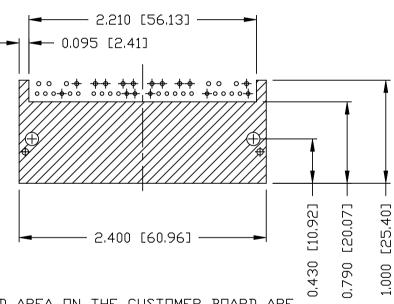
THE SHADED AREA ON THE CUSTOMER BOARD ARE RECOMMENDED TO BE CLEAR OFF ANY VIA HOLE OR COMPONENT PAD.
