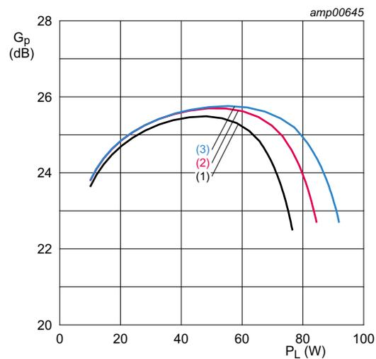
$I_{Dq} = 2 \times 25 + 2 \times 50$  mA;  $T_{mb} = 25$  °C;  $f = 2450$  MHz.
