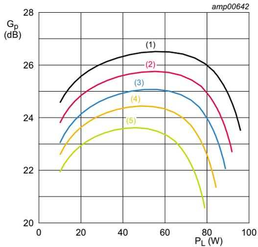
$I_{Dq} = 2 \times 25 + 2 \times 50$  mA;  $V_{DS} = 32$  V;  $f = 2450$  MHz.
