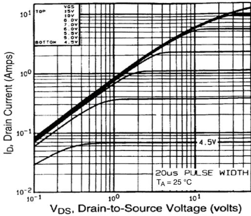
Fig. 1 - Typical Output Characteristics,  $T_A = 25\text{ °C}$
