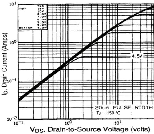
Fig. 2 - Typical Output Characteristics,  $T_A = 150\text{ °C}$
