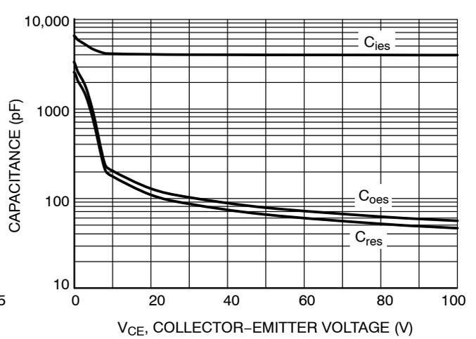
Figure 6. Typical Capacitance
