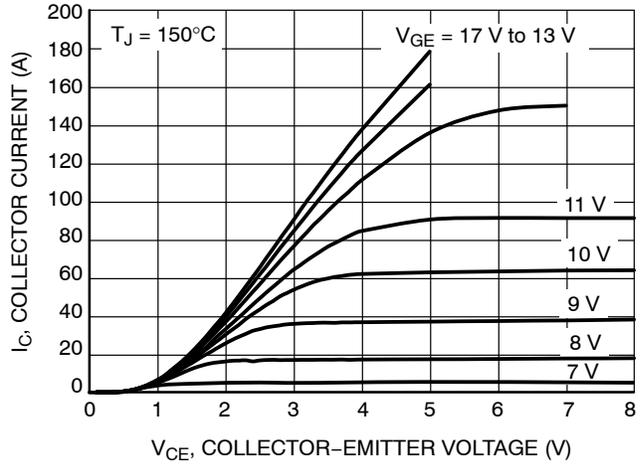
Figure 2. Output Characteristics
