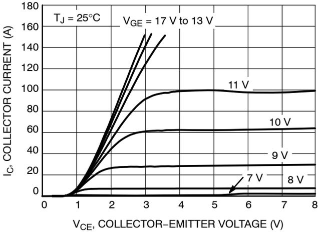
Figure 1. Output Characteristics
