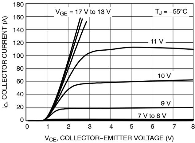
Figure 3. Output Characteristics
