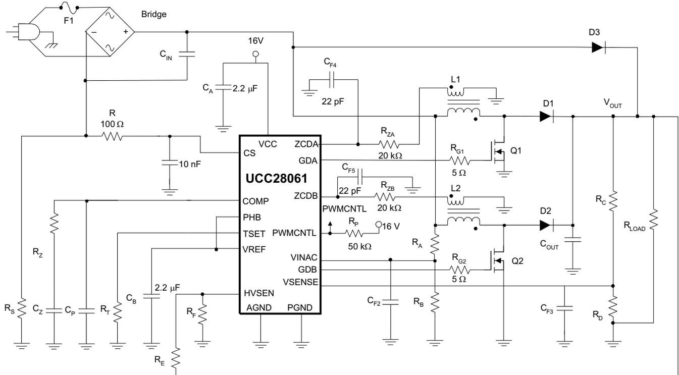
Figure 28. Typical Transition Mode Interleaved PFC Pre-Regulator
