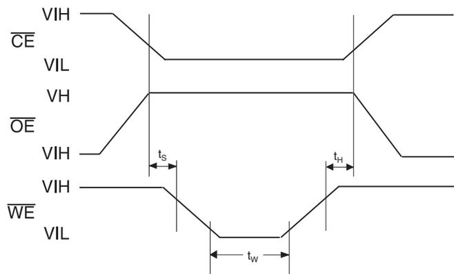
$t_s = t_h = 5 \mu\text{s}$  (min.)
