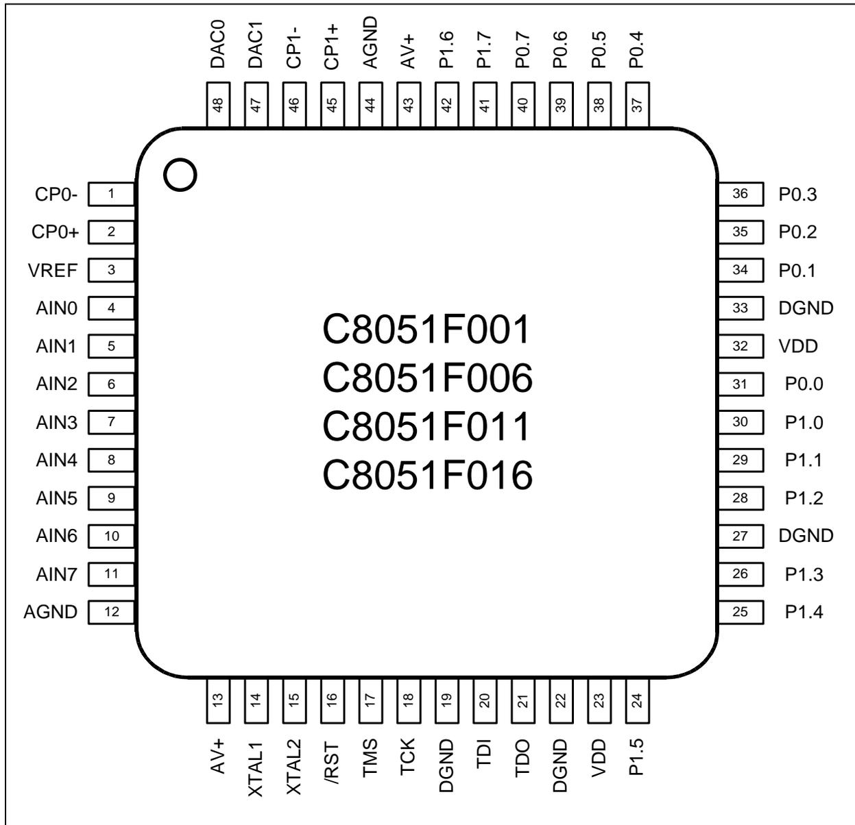
Figure 4.4. TQFP-48 Package Drawing
