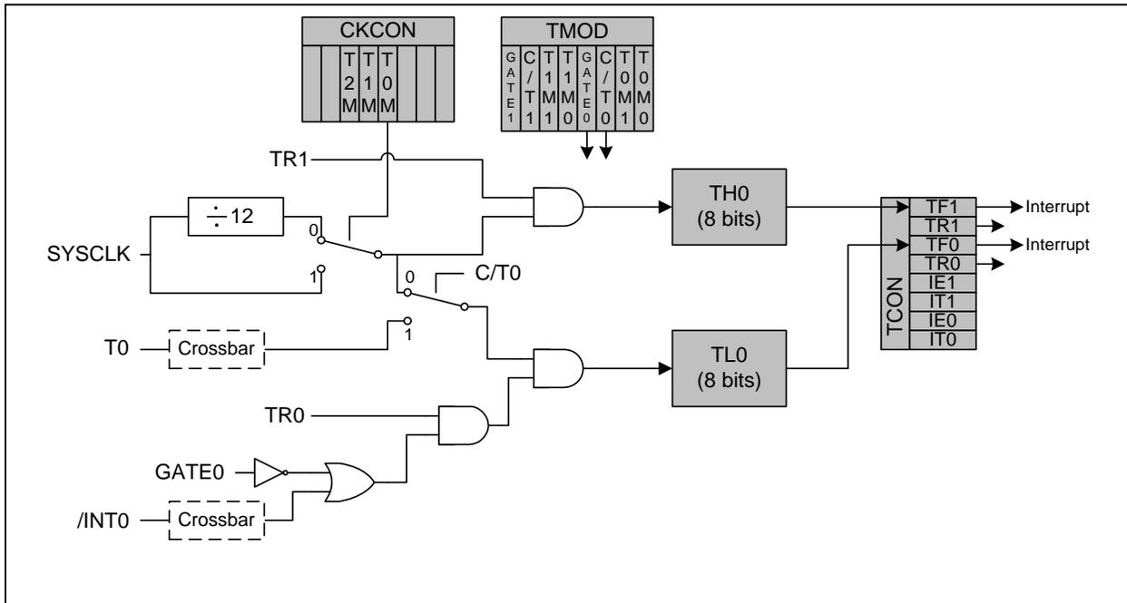
**Figure 19.4. TCON: Timer Control Register**
