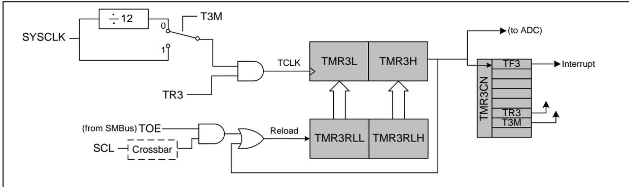
**Figure 19.20. TMR3CN: Timer 3 Control Register**
