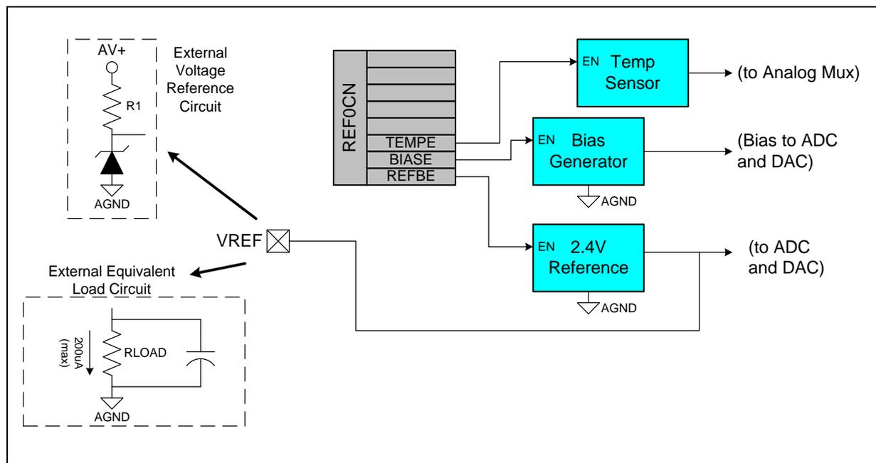
**Figure 9.2. REF0CN: Reference Control Register**
