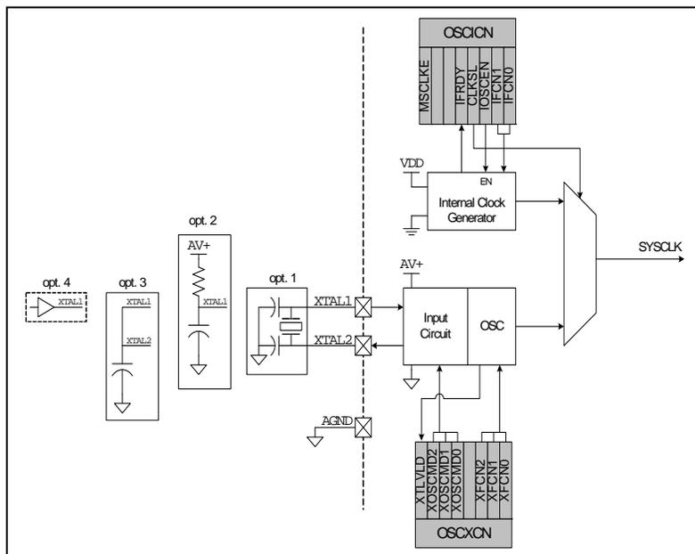
**Figure 14.2. OSCICN: Internal Oscillator Control Register**
