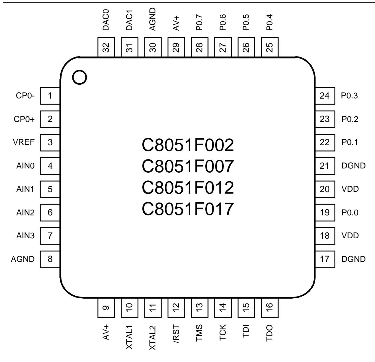
Figure 4.6. LQFP-32 Package Drawing
