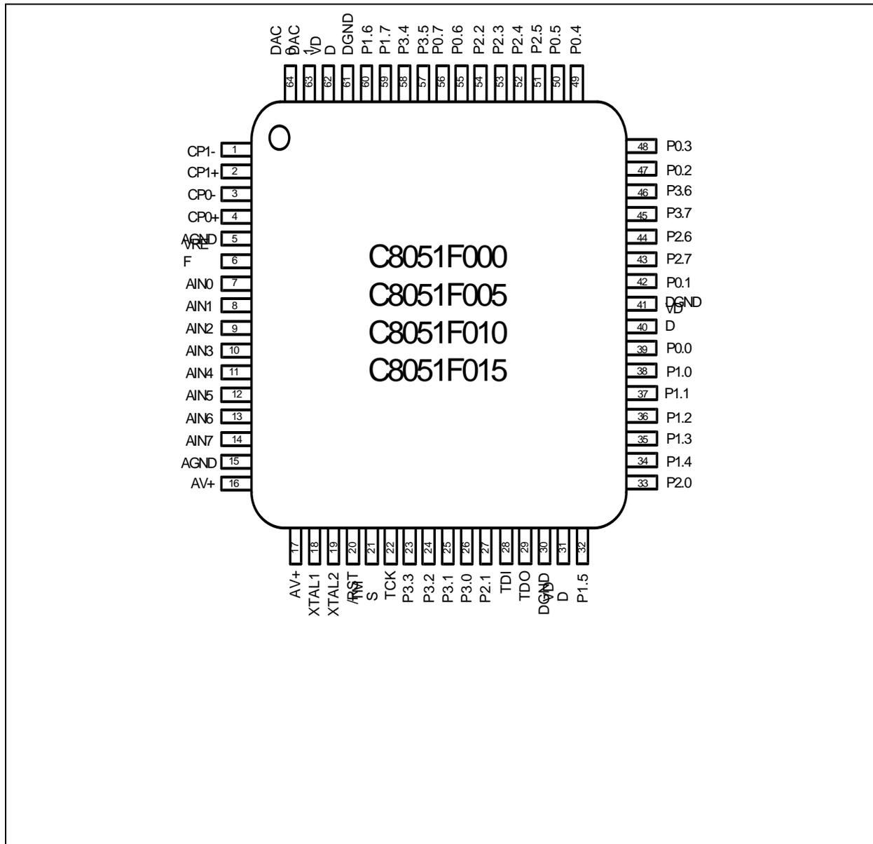
Figure 4.2. TQFP-64 Package Drawing
